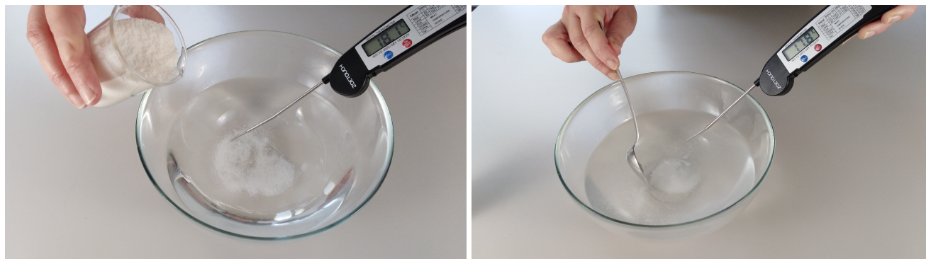
FIG. 6: (Colors online). The execution of the first part of the hands-on activity. (Photo on the left) Measuring the initial temperature of the water and then starting pouring salt in it. (Photo on the right) Stirring the water with a spoon in order to dissolve the salt and, at the same time, measuring the temperature at all times. The temperature decreases by one or two Celsius degrees.
