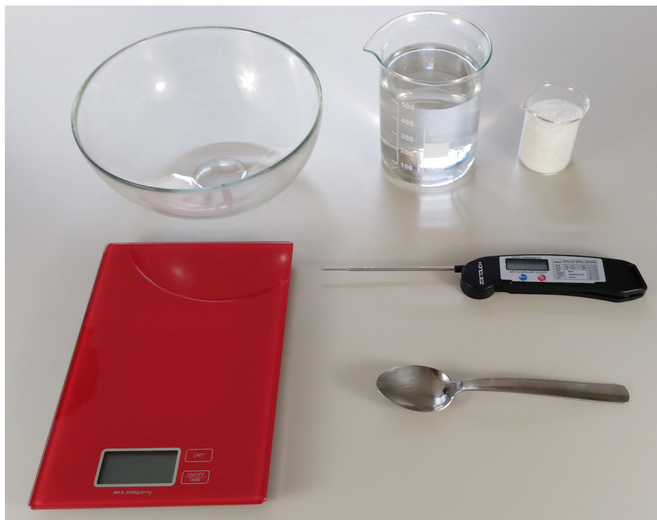
FIG. 5: (Colors online). The material for the first part of the hands-on activity. From the top left, in clockwise order: a large bowl, a beaker with 500 mL of room-temperature water, about 100 g of kitchen salt (NaCl), a thermometer, a rod or a spoon to stir the water, a scale.
