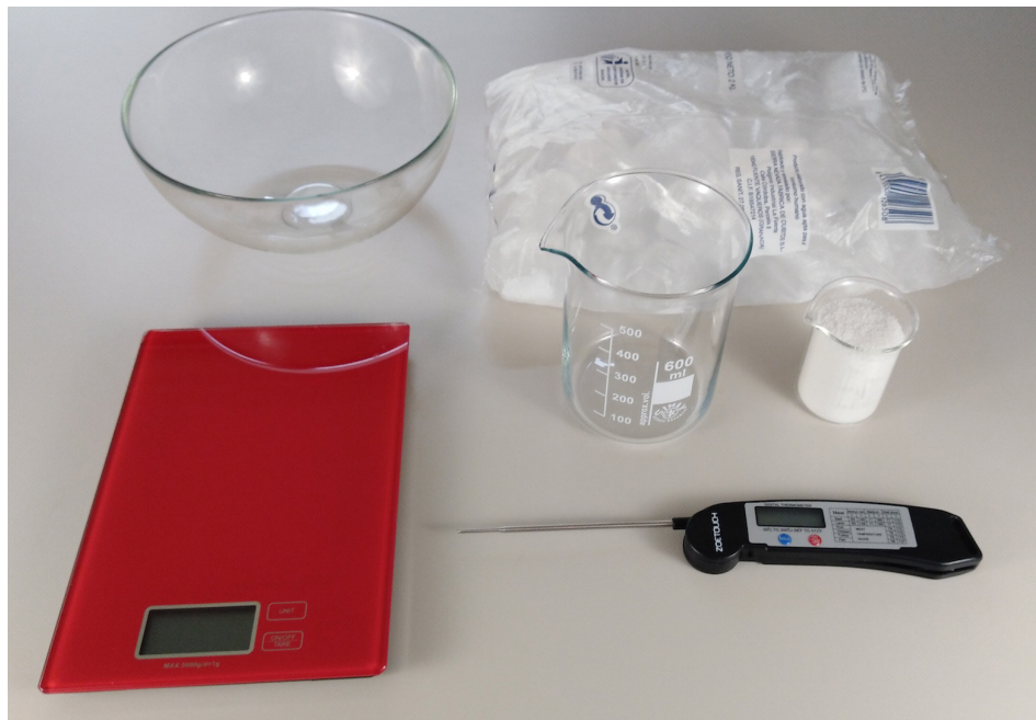
FIG. 7: (Colors online). The material for the second part of the hands-on activity. From the top left, in clockwise order: a large bowl, a bag of ground ice (at least 400 g), a beaker with 500 mL of room-temperature water, about 100 g of kitchen salt ( \text{NaCl} ), a thermometer, a rod or a spoon to stir the water, a scale.
