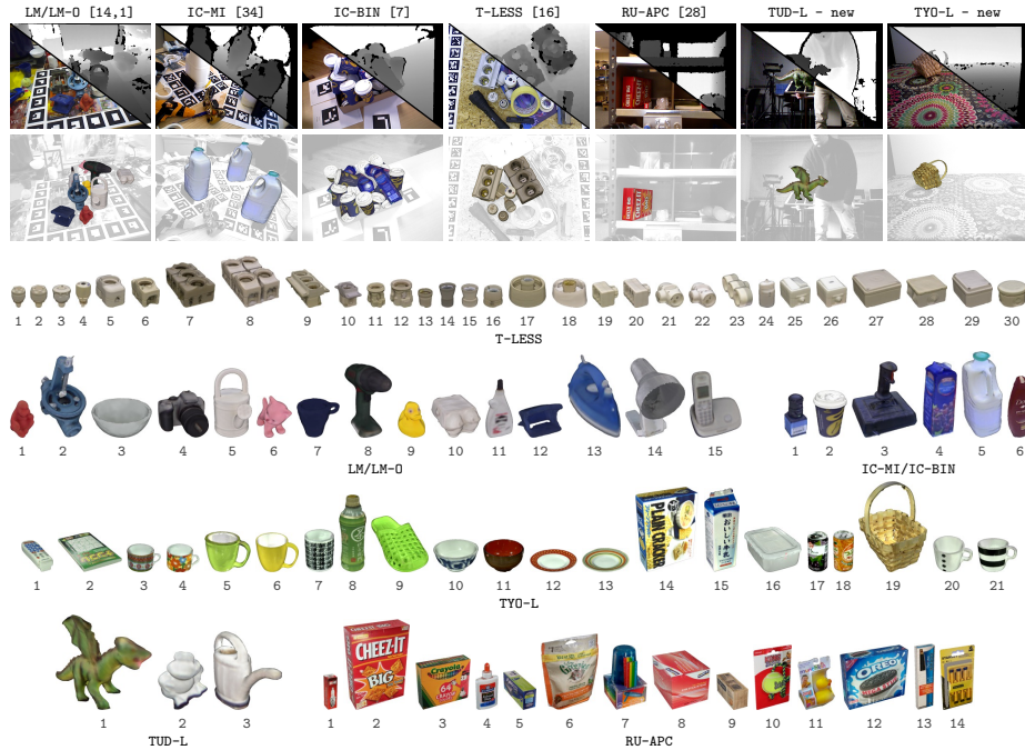
Fig. 1. A collection of benchmark datasets. Top: Example test RGB-D images where the second row shows the images overlaid with 3D object models in the ground-truth 6D poses. Bottom: Texture-mapped 3D object models. At training time, a method is given an object model or a set of training images with ground-truth object poses. At test time, the method is provided with one test image and an identifier of the target object. The task is to estimate the 6D pose of an instance of this object.
