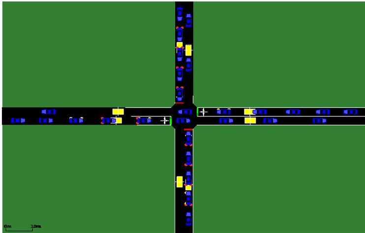
Figure 2: Intersection used for evaluating the detector. Yellow rectangles represent induction-loop sensors.
