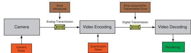
Fig. 1. Noise and error model for video broadcasting and surveillance systems
