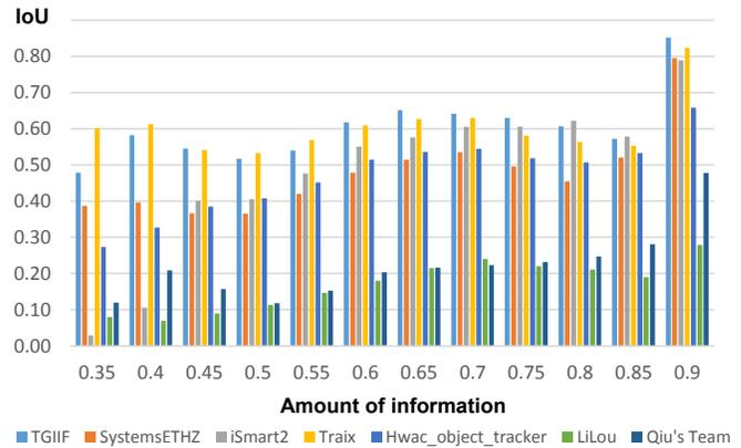
Fig. 20. Detection accuracy of FPGA entries with respect to amount of information.
