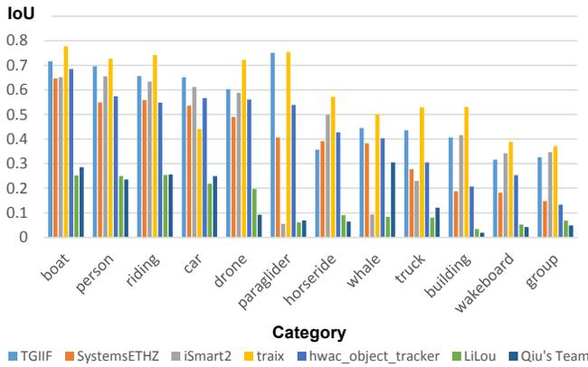
Fig. 17. Detection accuracy of FPGA entries with respect to image categories. Note that the category is sorted in a ranked order and the left-most one is with the highest average total score.
