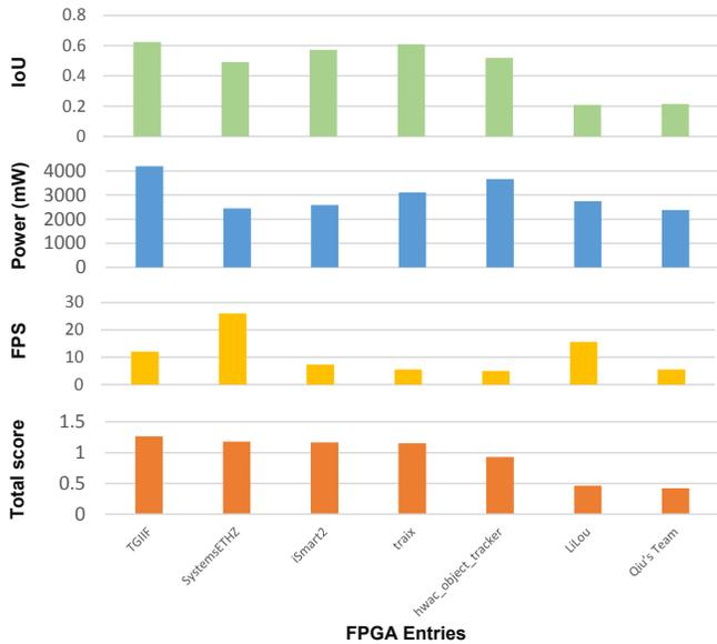
Fig. 15. Overall results of FPGA entries. The details of the scores can be found on the website of the challenge.
