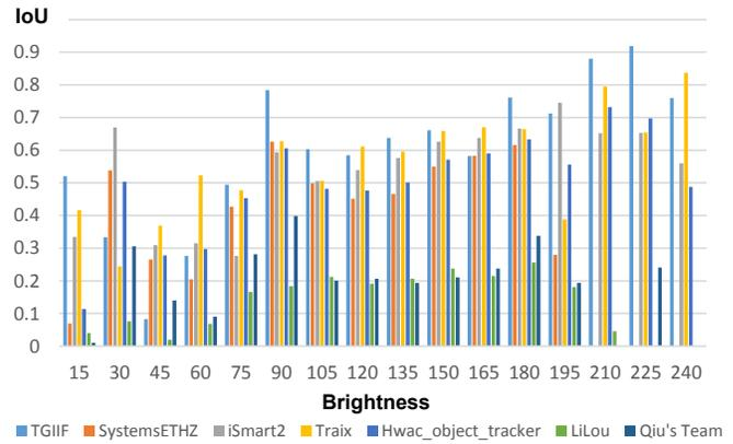
Fig. 19. Detection accuracy of FPGA entries with respect to brightness.
