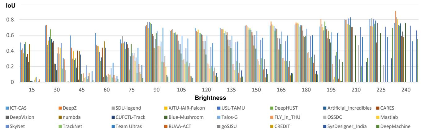
Fig. 13. Detection accuracy of GPU entries with respect to brightness.
