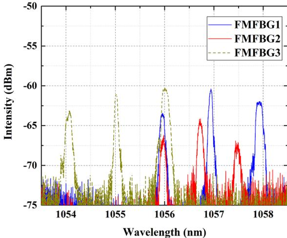
**Fig. 2.** The reflection spectra of the FMFBGs
