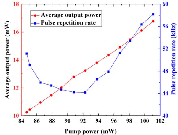
**Fig. 4.** The average output power and the pulse repetition rate of the Q-switching pulse versus the pump power.
