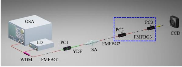
**Fig. 1.** Schematic illustration of the Q-switching CVB fiber laser.
