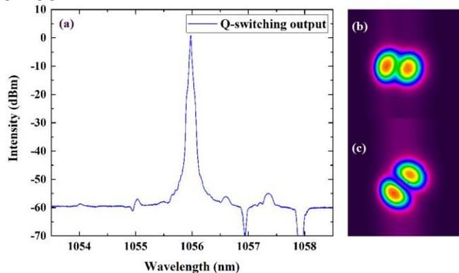
Fig. 5. (a) The optical spectrum of the laser from the pass port of the WDM; (b) the intensity profile of the output beam without the FMFBG3; (c) the intensity profile of the output beam after the FMFBG3.
