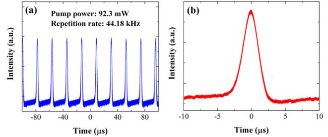
**Fig. 3.** (a) The Q-switching pulse train and (b) single pulse envelope under the pump power of 92.3 mW.
