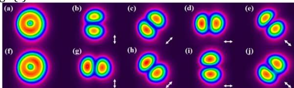
Fig. 6. (a) Beam profile of radial mode without a linear polarizer; (b)–(e) Transmitted intensity distributions of radial mode after a linear polarizer; (f) Beam profile of azimuthal mode without a linear polarizer; (g)–(j) Transmitted intensity distributions of azimuthal mode after a linear polarizer. The white arrows indicate the corresponding axis of the polarizer.
