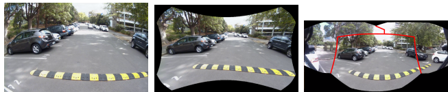
Fig. 5: Demonstration of one frame from the center camera being inserted into the panorama image. The left image is the original image, the center image is after undistortion, and the right image is after the image has been warped and inserted into a panorama canvas with the other two camera images. The edges of these image have been highlighted for clarity.
