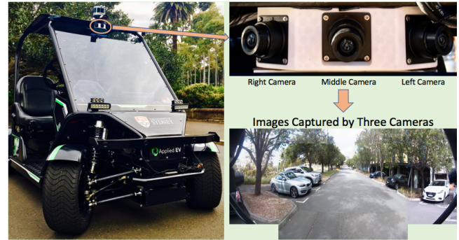
Fig. 1: Autonomous electrical vehicle. There are three NVIDIA GMSL cameras mounted in the front of the vehicle. Images captured by these three cameras can cover a 180° field of view. Two side cameras have around 20° overlap. The middle camera is tilted 15° downwards.
