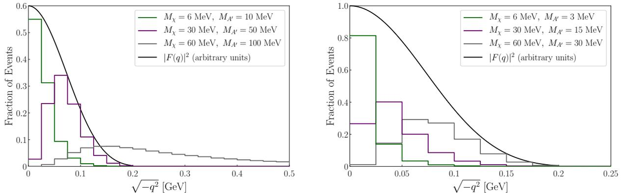
FIG. 5. The distribution of the momentum transfer to the argon nucleus for six dark matter and dark photon mass combinations. The dark matter to dark photon mass ratio is set to 0.6 (2) in the left (right) plot. The black curves in the same plots show the Helm form factor  $F(q^2)$ . In the left plot  $F(q^2)$  has been scaled by 0.6 for clarity.
