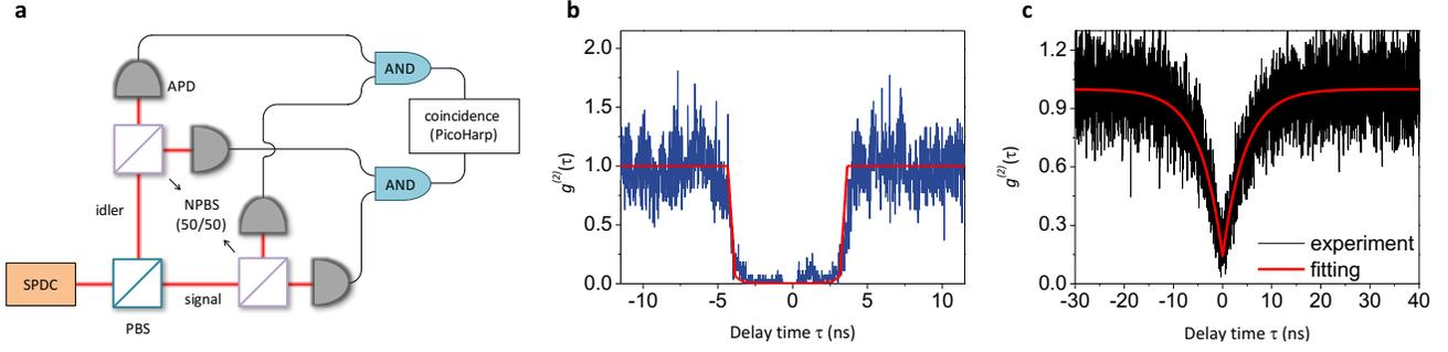
FIG. 4. **Second order correlation function of the resources.** **a**, Experimental schematic for measuring the anti-bunching property of heralded single photons [39, 40]. **b**, Experimental (blue line) and theoretical values (red line) of the second order correlation function of heralded single photons. Average value of  $g^{(2)}$  dip is 0.036. **c**, The  $g^{(2)}(\tau)$  function of single photons emitted from a single terrylene molecule. The result reads  $g^{(2)}(0) = 0.14$ .
