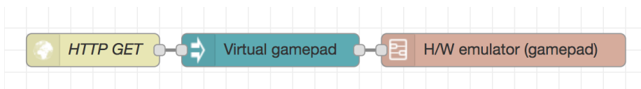
Fig. 7. Visual programming example for pressing a gamepad button after receiving an HTTP GET request.
