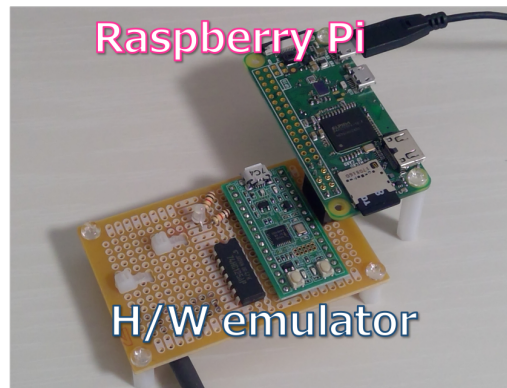
Fig. 4. (Left) H/W emulator and (right) Raspberry Pi Zero W, which runs the visual programming element.
