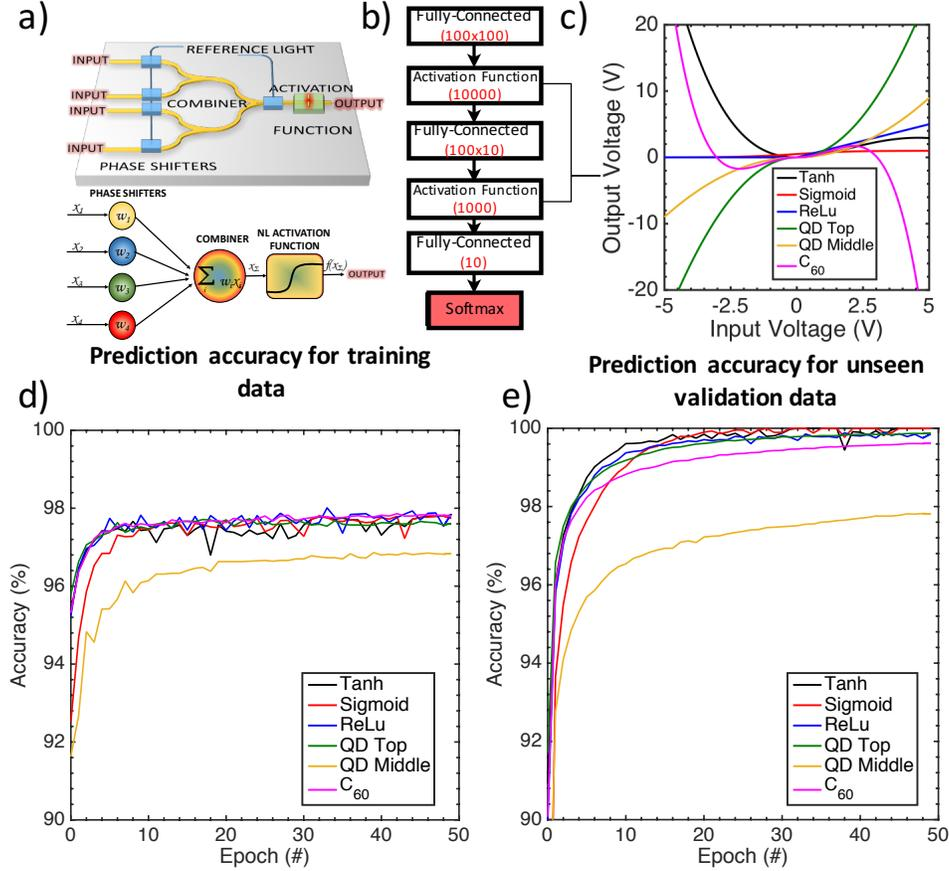
Fig. 5. Design of an AO neuron and evaluation of the Neural Network performance a) Schematic of an all-optical neuron. b) Representation of the emulated NN (b). c) Different activation functions,  $V_{IN}$  to  $V_{OUT}$ , ReLU (light blue dashed line), Sigmoid (blue dashed line), hyperbolic tangent (dark blue line) and the 2 proposed NL function, top (solid orange) and middle (solid red) d-e) Prediction accuracy as function of epoch for the training (d) and validation (e) phase of the network.
