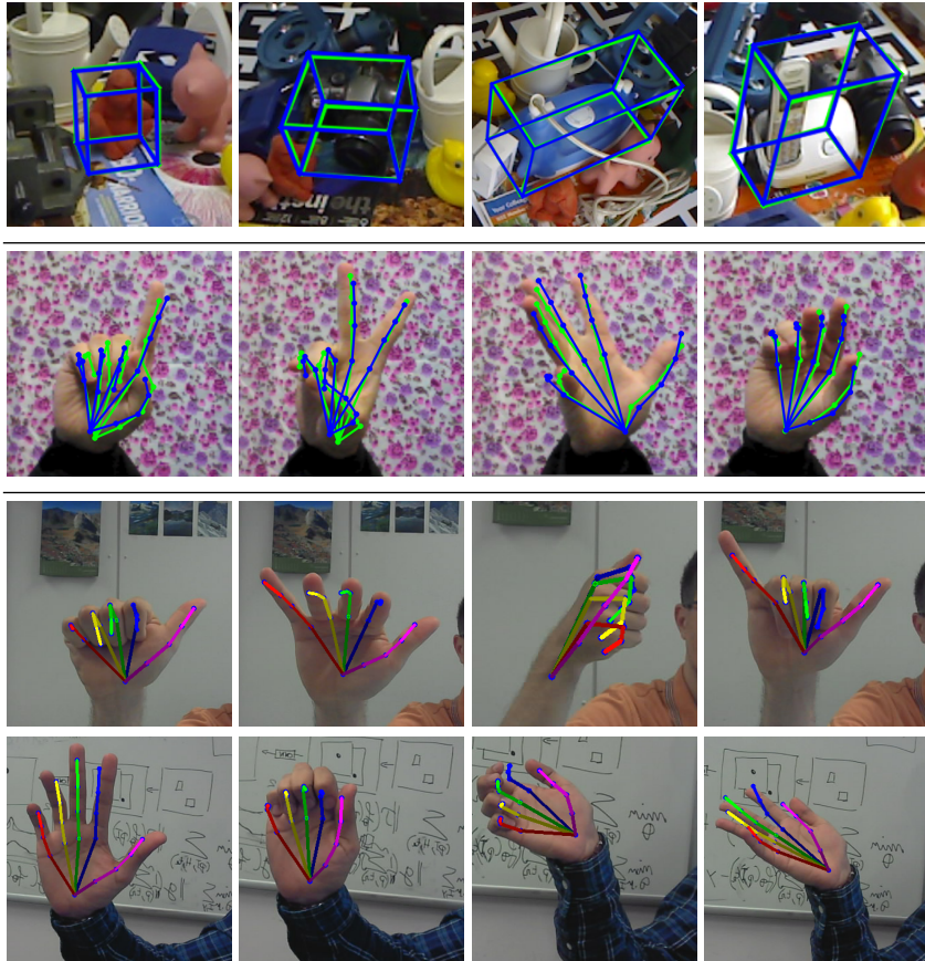
Fig. 6: Qualitative results of our method for 3D rigid object pose estimation on the LINEMOD dataset [6] (top row), and 3D hand pose estimation on the STB dataset [18] (middle row). Green denotes ground truth and blue corresponds to the predicted pose. We applied our trained network on real world RGB images of different users to estimate the 3D hand joint locations (bottom rows).
