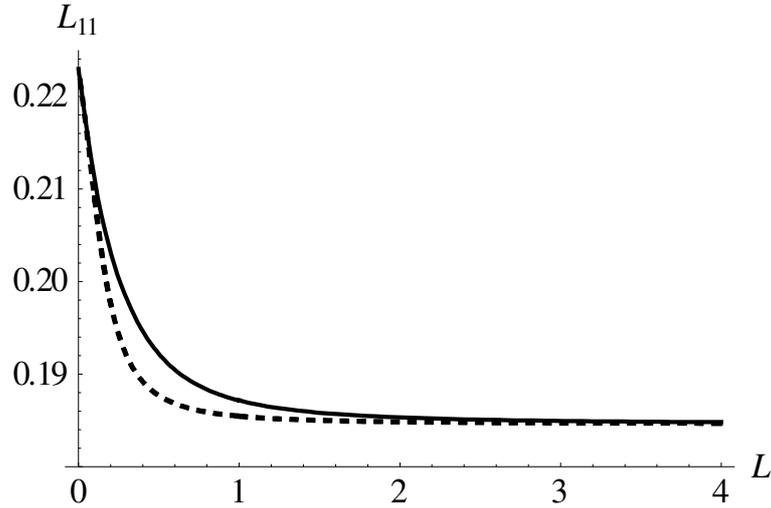
**Fig.4.** Variation of hydrodynamic permeability with scale parameter  $L$  under no couple stress condition (solid line) and no spin condition (dashed line) on the outer surface of the cell.
