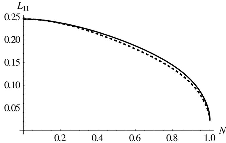
**Fig.3.** Variation of hydrodynamic permeability with coupling parameter  $N$  under no couple stress condition (solid line) and no spin condition (dashed line) on the outer surface of the cell.
