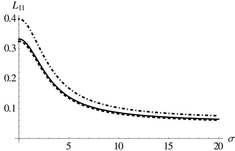
**Fig.6.** Variation of hydrodynamic permeability with parameter  $\sigma$  under no couple stress condition (solid line), no spin condition (dashed line) on the outer surface of the cell and for the Newtonian liquid (dot-dashed line).
