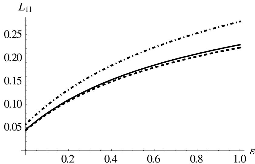
**Fig.7.** Variation of hydrodynamic permeability with porosity  $\varepsilon$  under no couple stress condition (solid line), no spin condition (dashed line) on the outer surface of the cell and for the Newtonian liquid (dot-dashed line).
