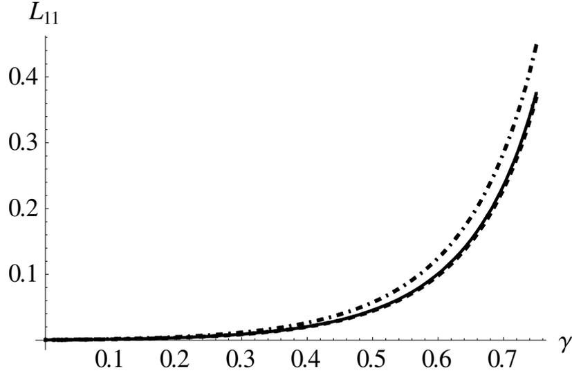
**Fig.8.** Variation of hydrodynamic permeability with porosity  $\gamma$  under no couple stress condition (solid line), no spin condition (dashed line) on the outer surface of the cell and for the Newtonian liquid (dot-dashed line).
