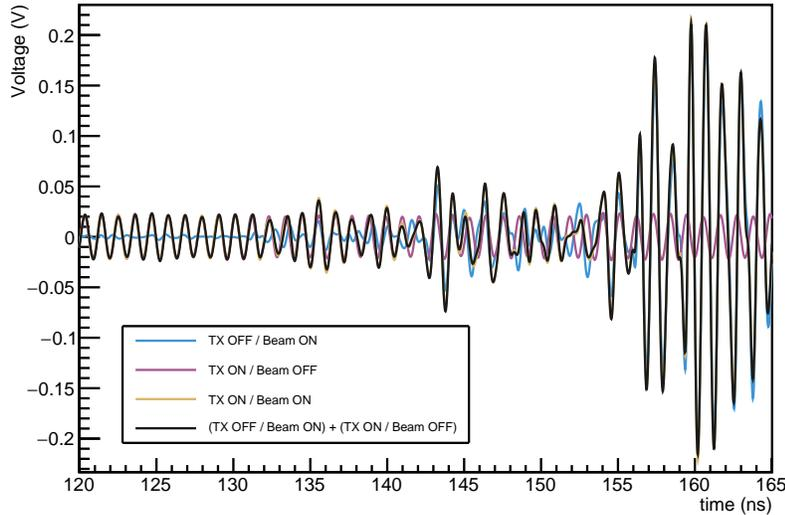
FIG. 7: An example of ‘null’ data construction. A carrier-only (TX ON / Beam OFF) event is phase aligned with the carrier of a real event, and a beam-only (TX OFF/ Beam ON) event is phase aligned with the beam splash of a real event. The two are summed to produce an event which mimics real events in phase and amplitude.
