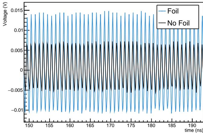
FIG. 4: A ‘foil test’, for which a conductor (here  $0.3 \text{ m} \times 1 \text{ m}$ ) is placed at the expected ionization maximum point on the target, to estimate how a reflection should be observed in the receiver. In this test, the foil reflection is in phase with the ambient background, indicating a good receiver position.
