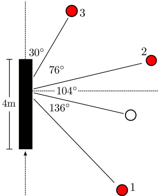
FIG. 3: The setup for run 11 of T576, viewed from above, and drawn to scale. Closed circles are receivers, labeled by their DAQ channel number, open circle is the transmitter. One receiver is at the specular reflection point relative to calculated shower maximum; the others are separated from the specular angles by 30–40 degrees.
