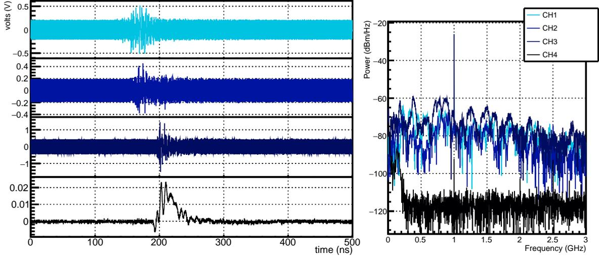
FIG. 5: A typical T576 event. The 4 left panels are channels 1-4 from top to bottom, respectively, and the right panel shows their associated PSD. The offsets on the x-axis are due to air and cable propagation delays.
