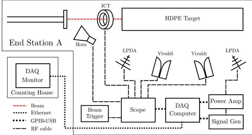
FIG. 2: The T576 signal chain. The DAQ system and transmitter resided in the End Station A, and were remotely monitored via an Ethernet link from the ‘counting house’, a remotely accessible location for users while the beam is on. The various components shown are described in the text.
