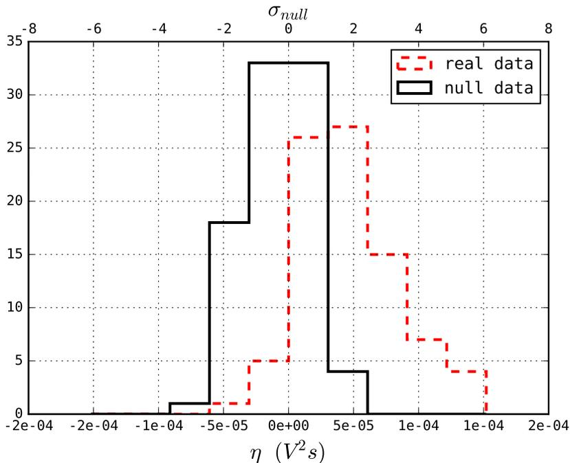
FIG. 19: The significance of the signal using the 2D sideband subtraction routine. X axis units are given in  $V^2s$  and also in terms of standard deviations of the null data distribution, denoted  $\sigma_{null}$ .
