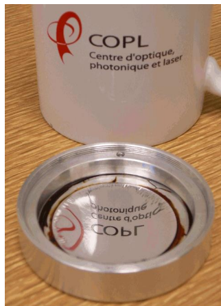
Figure 3. Ferrofluidic mirror covered with an elastomer membrane coated with a thin layer of aluminum.
