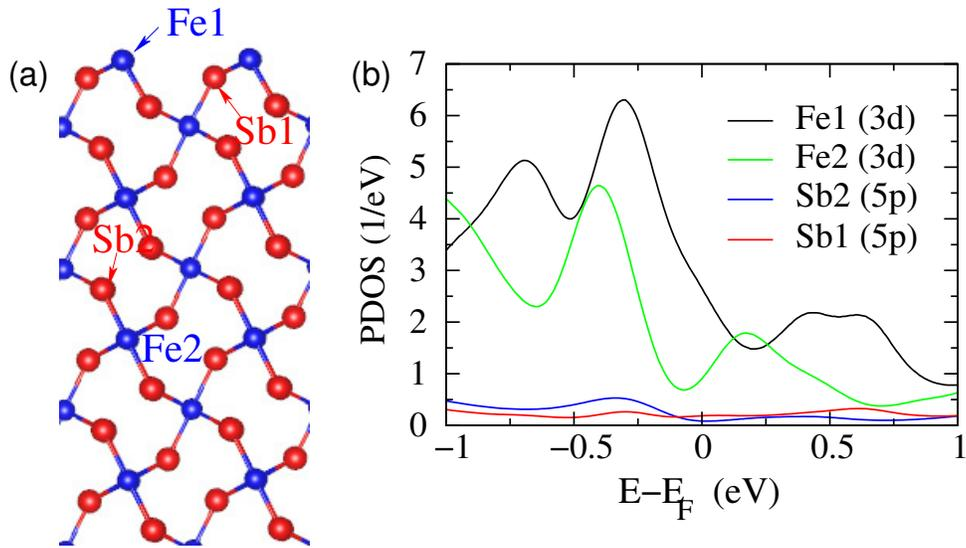
Figure 8: (a) Theoretical slab model for the FeSb<sub>2</sub> surface which is terminated in Fe (blue spheres). (b) Projected density of states on the Fe1, Fe2, Sb1, and Sb2 sites illustrated in (a).
