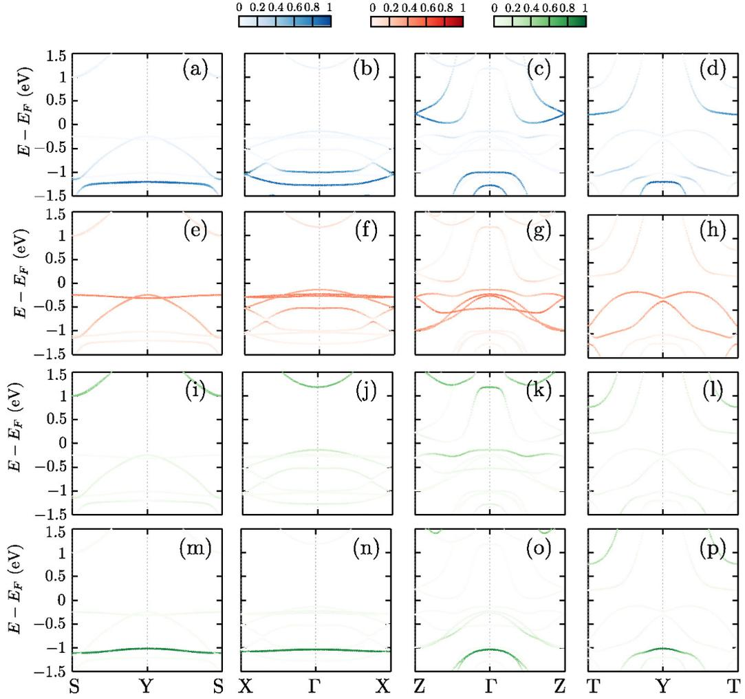
Figure 7: Fe-3d orbital resolved LQSGW band structure along the same high-symmetry directions in BZ as ARPES data. Projections to Fe- $d_{xy}$  (a-d), Fe- $d_{yz}/d_{xz}$  (e-h), Fe- $d_{z^2}$  (i-l), and Fe- $d_{x^2-y^2}$ , are shown in blue, red, and green, respectively.
