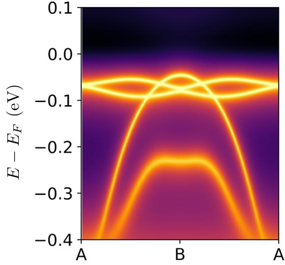
Figure 10: LQSGW+DMFT spectral function of FeSb<sub>2</sub> bulk along A-B-A at 50 K.
