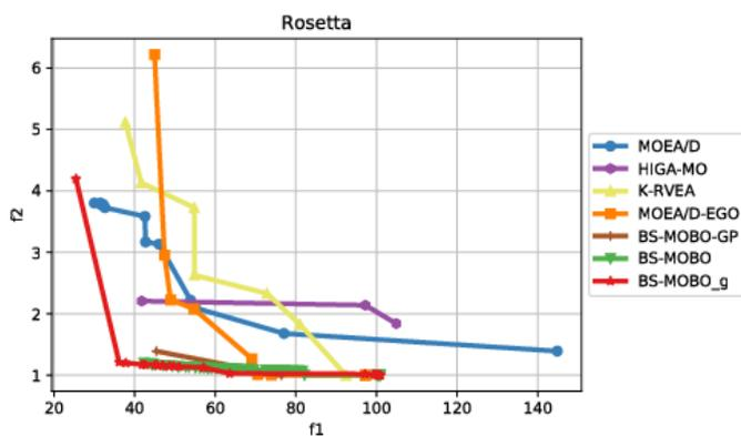
Fig. 8. The approximated Pareto front obtained by different algorithms on the Rosetta problem.
