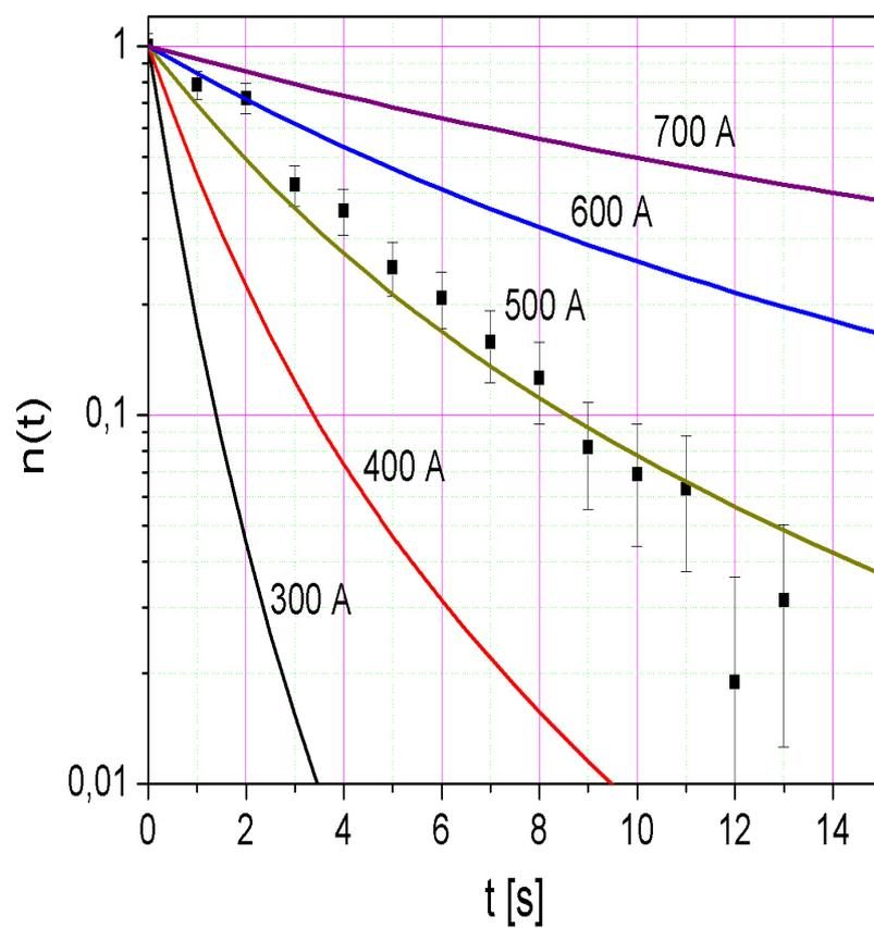
Рис. 8: Dots represent the results of measurements of the UCN storage curve in the titanium chamber. Curves were calculated for different thicknesses of the  $\text{TiO}_2$  film.
