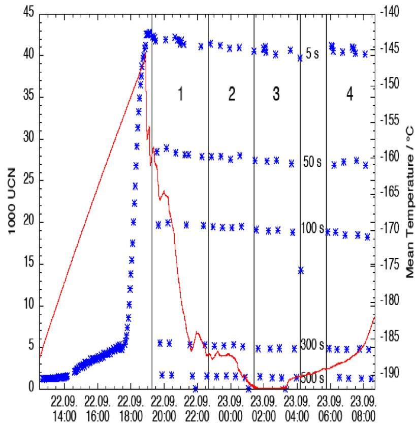
Рис. 4: Temporal pattern of UCN storage in the fluoropolymer-coated chamber. The curve represents the variation of temperature with time (right scale). Dots correspond to the numbers of neutrons remaining after 5, 50, 100, 300, and 500 s (left scale). The astronomical measurement time is indicated on the horizontal scale.
