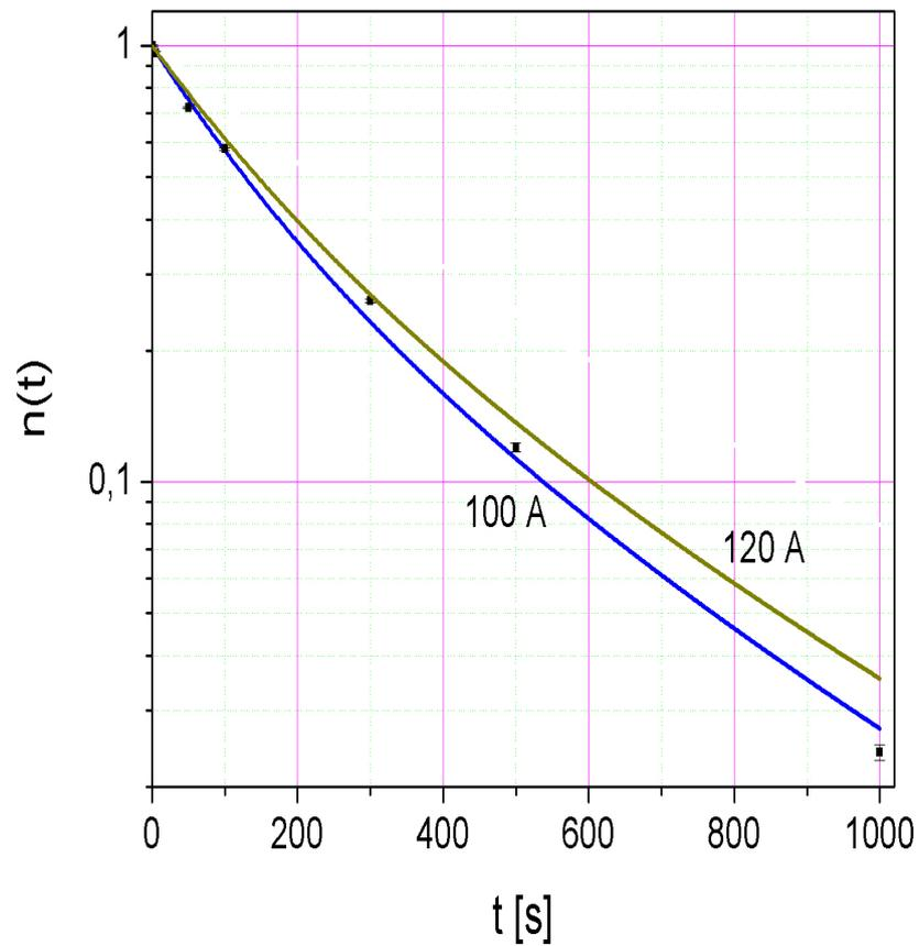
Рис. 11: Measured data on the UCN storage in the fluoropolymer-coated chamber (dots) and storage curves modelled with an assumed fluoropolymer thickness of 650 Å and two different thicknesses of the TiO<sub>2</sub> film (100 and 120 Å).
