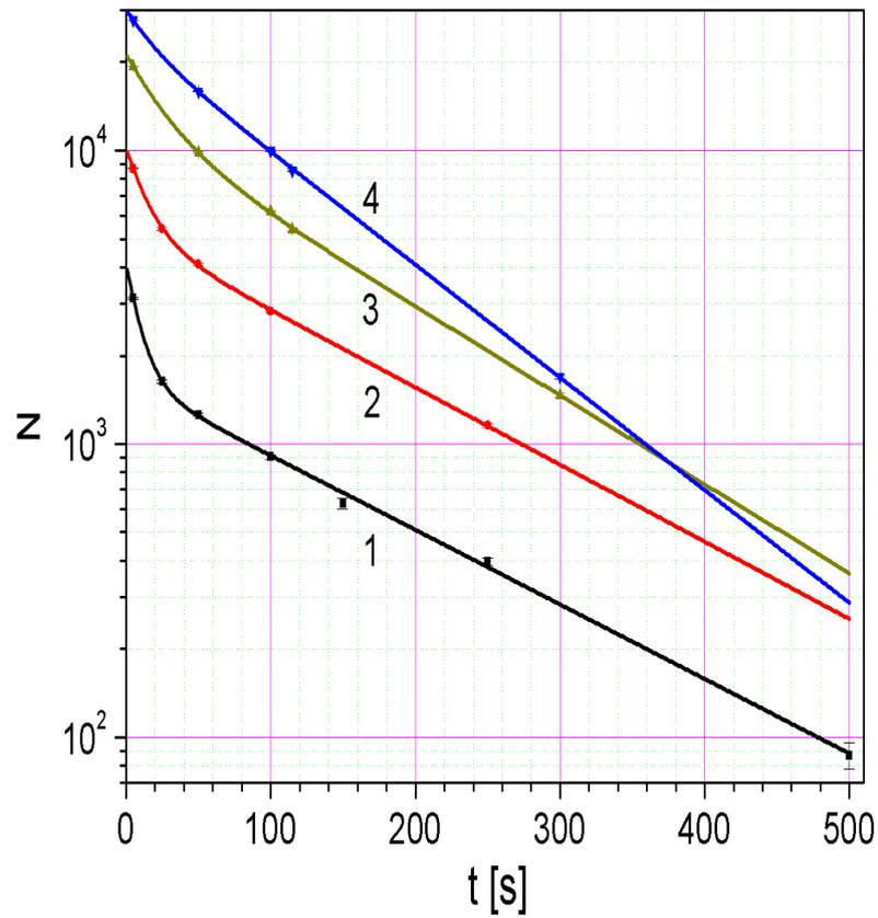
Рис. 6: Measured UCN storage curves in the fluoropolymer-coated chamber with a boron absorber located at a height of 31 (1), 50(2), 75 (3), or 100 cm (4). The approximating curves were obtained in a double-exponential model.
