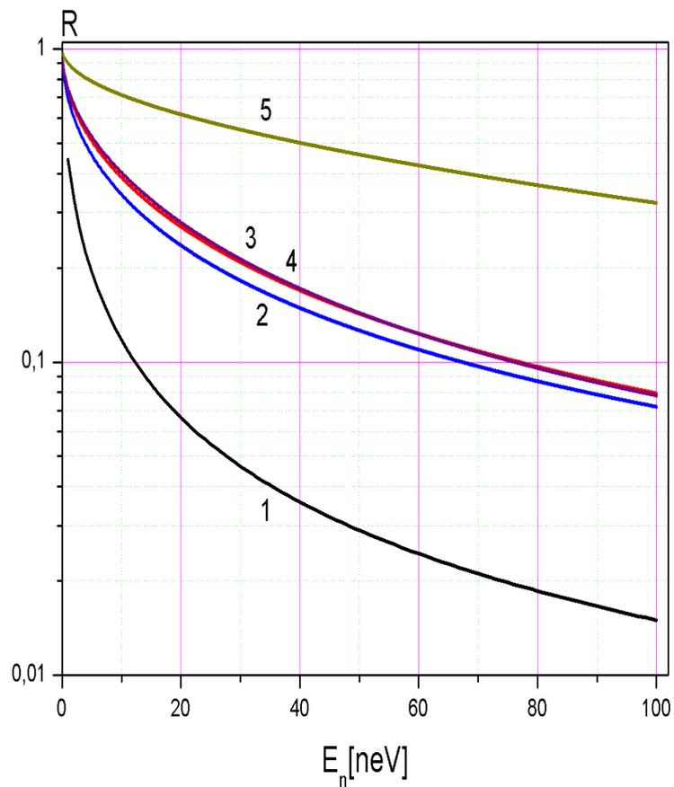
Рис. 5: Calculated coefficients of reflection of neutrons incident isotropically onto the surface of several absorbers: polyethylene (1), titanium (2),  $^{10}\text{B}$ , and  $^{10}\text{B}_{0.94}\text{B}_{0.06}$  (3, 4), and gadolinium (5).
