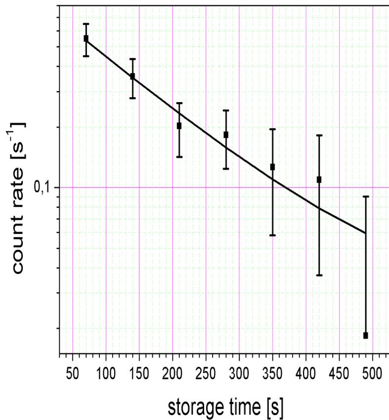
Рис. 10: Temporal variation of the count rate of the side boron counter measured in experiments performed in the fluoropolymer-coated chamber. The curve is the result of approximation with a single exponential model.
