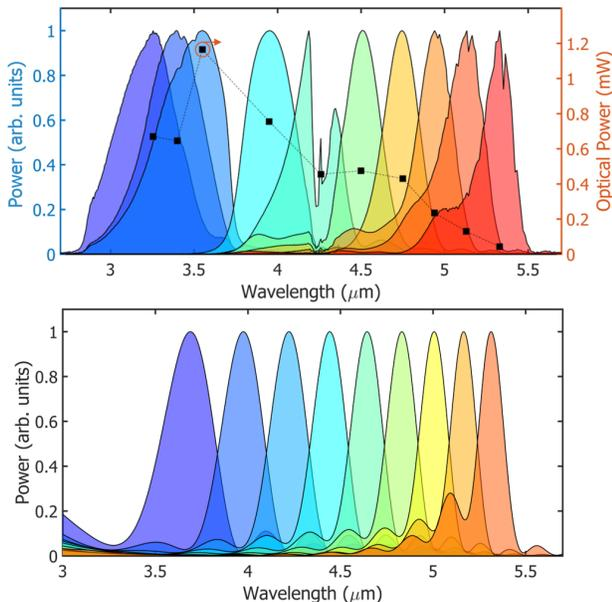
FIG. 2. MIR Spectra. (a) Experimentally measured intra-pulse DFG spectra. Measured with a commercial FTS (4  $\text{cm}^{-1}/120$  GHz resolution). All spectra are normalized, with measured power indicated by the square markers. Atmospheric  $\text{CO}_2$  absorption is visible in the spectrum centered around 4.2  $\mu\text{m}$ . (b) Predicted MIR spectra, also normalized.
