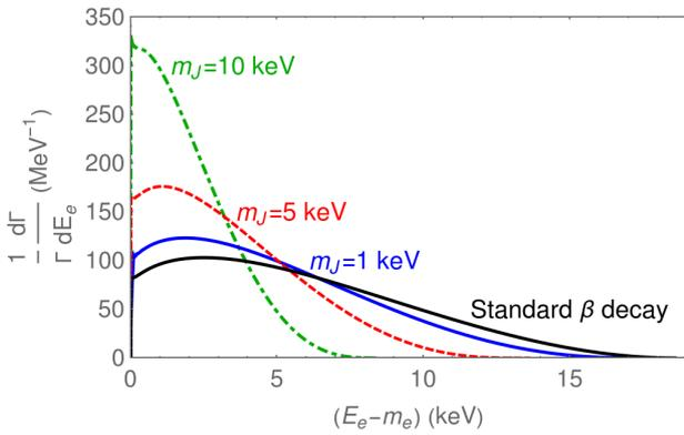
FIG. 1. Normalized electron energy spectrum of the decay  ${}^3\text{H} \rightarrow {}^3\text{He}^+ + e^- + \bar{\nu}_e + J$  (with the pseudoscalar  $J$  emitted from the neutrino) and the standard  $\beta$ -decay spectrum. The coupling  $g_{\nu J}$  has been set to 1, the spectrum scales with  $g_{\nu J}^2$ .
