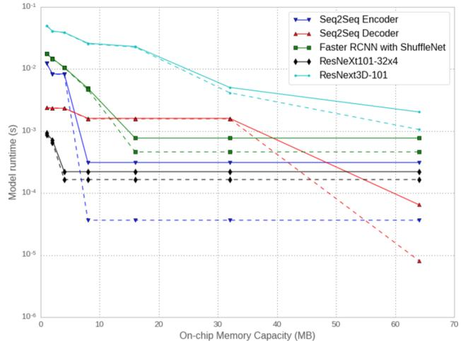
**Figure 3: Runtime roofline analysis of different DL models with parameters stored as int8 numbers on a hypothetical accelerator with 100 TOP/s and 100 GB/s DRAM bandwidth. The performance is shown for varying on-chip memory capacity with 1 TB/s (solid) and 10 TB/s (dashed) bandwidth.**
