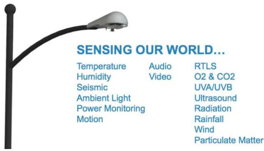
Fig. 7. Different sensors for a street lighting in a smart city [18].
