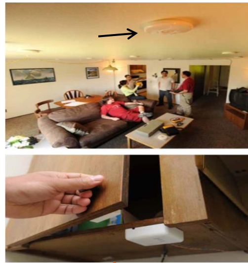
Fig. 2. Common ambient sensors monitor (top) infrared-based motion, ambient light, ambient temperature and (bottom) door open/close status. Arrows indicate a sensor location [11].
