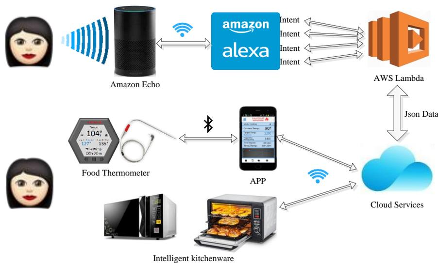
Figure 1. Smart Cooking Architecture based on Amazon Echo
