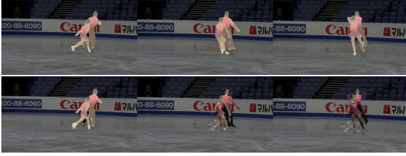
Figure 5: Top: JITNet 0.9 predictions on a sequence of three frames which are roughly 0.13 seconds apart (4 frames apart) in the Figure Skating video. Bottom: Large deformations, object and camera motion prove challenging to flow based interpolation.
