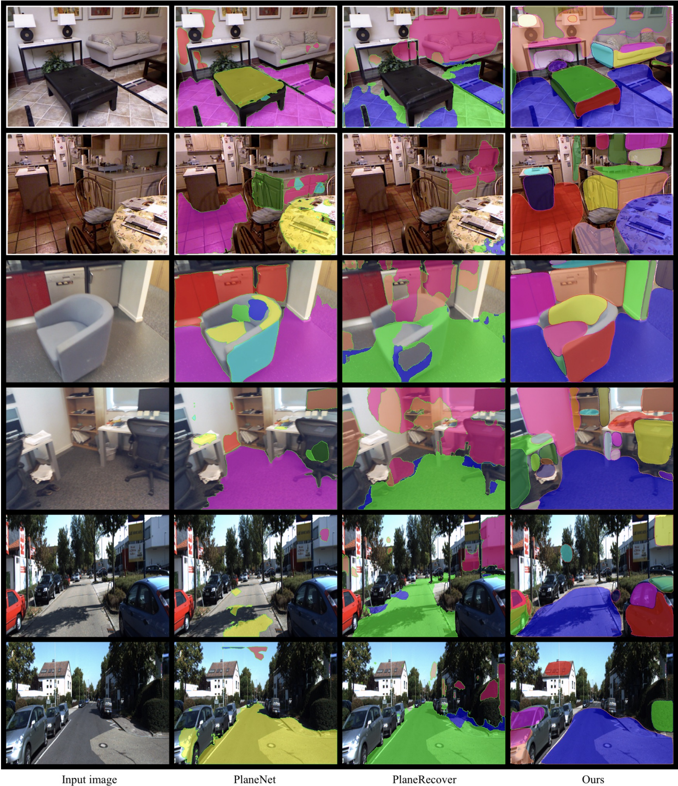
Figure 13. More plane segmentation results on unseen datasets without fine-tuning. From left to right: input image, PlaneNet [27] results, PlaneRecover [49] results, and ours. From top to the bottom, we show two examples from each dataset in the order of NYUv2 [37], 7-scenes [35], and KITTI [13].
