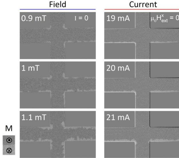
**FIG.8.** Kerr microscopy illustration of the initial stage of the Ru/Co/Ru/W Hall bar demagnetization under the action of the perpendicular field and current
