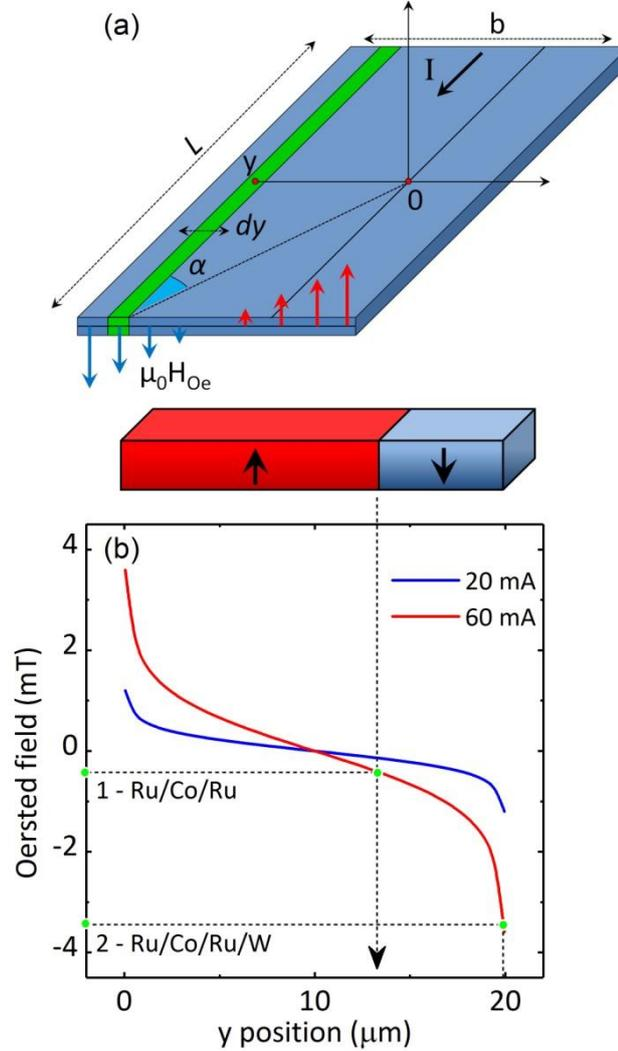
**FIG.7.** (a) Calculation scheme for the Oersted field on a homogeneous section of the Hall Bar. (b) The calculated distribution of the Oersted field in the cross section of the microstrip, perpendicular to the current direction. The vertical dashed lines mark the position of the domain wall for two structures after passing the maximum current into the presence of an external field  $\mu_0 H_{ext}^z = 8 \text{ mT}$
