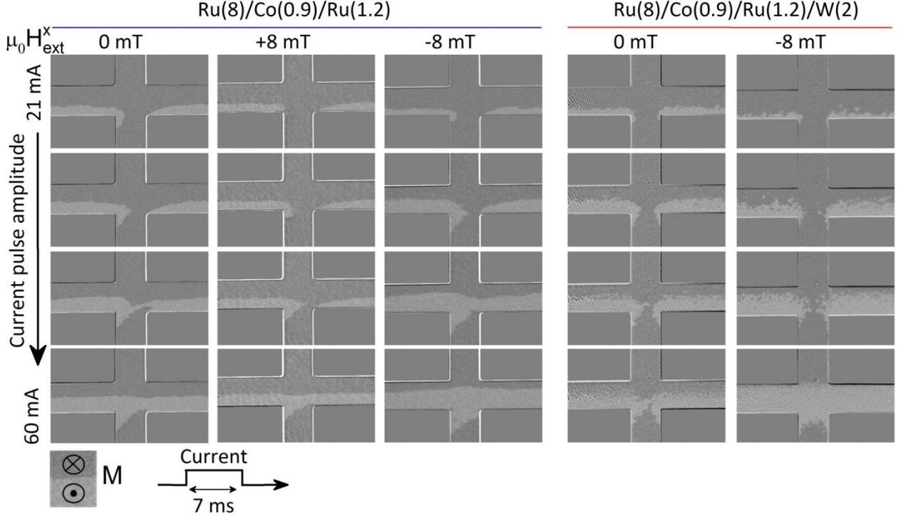
**FIG.4.** Changes in the domain structure during the current-induced magnetization reversal of Ru/Co/Ru and Ru/Co/Ru/W samples for different values of the field  $\mu_0 H_{ext}^x$
