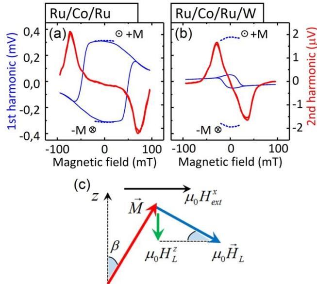
**FIG.5.** Dependence of the AHE amplitude on the magnitude of the in-plane field applied along the current direction at the first and second harmonics for structures without W (a) and with W (b). The signal at the first harmonic was also measured in a field range of  $\pm 20$  mT after the preliminary magnetization (dashed lines). (c) Scheme of mutual orientation of the magnetization, the effective field of SOT effect and its projection on z axis
