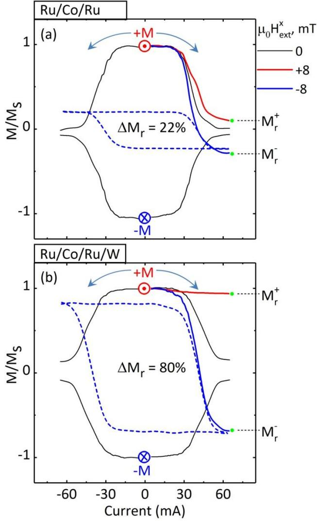
**FIG.3.** A set of demagnetization curves obtained by passing the current of increasing amplitude after preliminary magnetization to the saturation state with a different value of the in-plane field  $\mu_0 H_{ext}^x$  for the Ru/Co/Ru (a) and Ru/Co/Ru/W (b). Current-induced magnetic hysteresis loops allow determining of the switching amplitude
