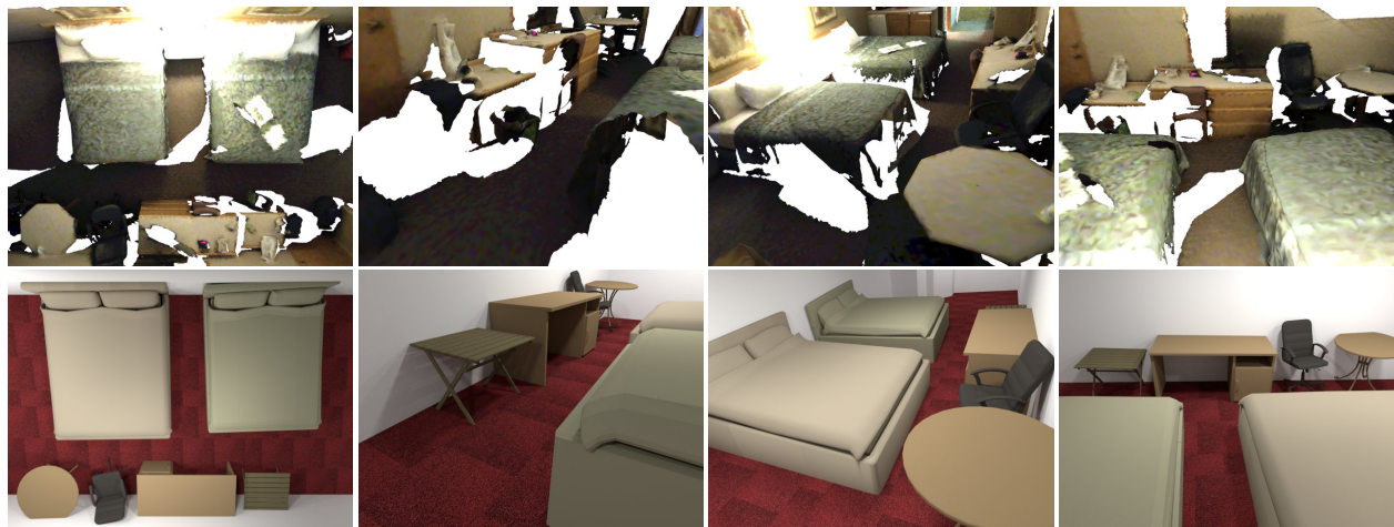
Figure 1. Given an RGBD sequence from a moving camera, we produce a 3D CAD recomposition of the scene. While a fused reconstruction (top) contains holes and noisy geometry, our recomposition (bottom) models the scene as a set of high quality 3D shapes from CAD databases.
