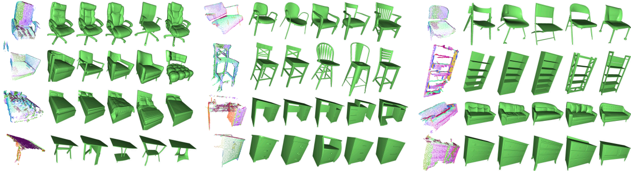
Figure 3. Top retrieved CAD models for each object instance segmentation as query. Point cloud query is color-coded with surface normal.
