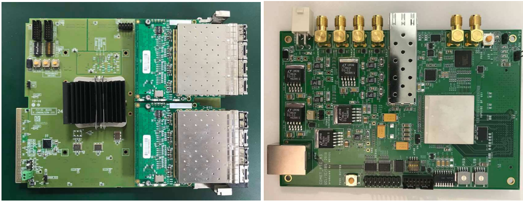
Figure 79: (Left) FC7 board developed for CMS experiment and adopted as the central trigger processor board in COMET trigger system. A FPGA for trigger processing and board control locates at the center, and two commercial mezzanine cards for connecting subdetector trigger system are mounted on the right side of the board. (Right) Custom-designed FCT board for interfacing with FC7 board.
