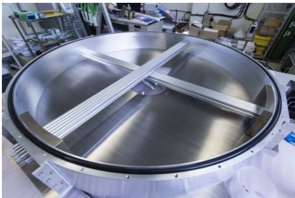
Figure 57: The Full-scale prototype, partially completed without the vacuum wall.
