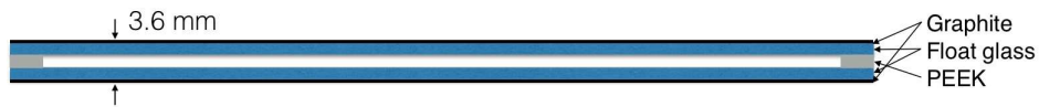
Figure 76: Single-gap GRPC made of two layers of float glass, glued together using 1.2 mm PEEK spacers. On the outer part of the glass sheets, a resistive painting (graphite-based) is used to apply an electric field of about 6.5 kV/mm across the gap. A mixture of a gas with high fluor content (forane) and a quencher ( SF_6 ) at a ratio of around 98:2 is flushed permanently through the chamber at a low rate of about 15 cc/min.
