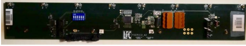
Figure 78: A Front End board, developed for ALICE, housing the FEERIC ASIC in the centre of the board. At the top, the eight pins connecting the readout strips (designed for 4.5 cm readout-strips in this case) are visible. The four pins on the bottom of the picture are for grounding. The board shown is 32.5 cm long and 5 cm wide, but the final dimensions will be determined by the optimal BS-CRV segmentation.
