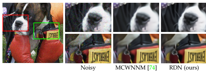
Fig. 14. Visual denoised results of the real noisy image “Dog”. The noise level of R, G, B channels are estimated as 16.8, 17.0, and 16.6 respectively.
