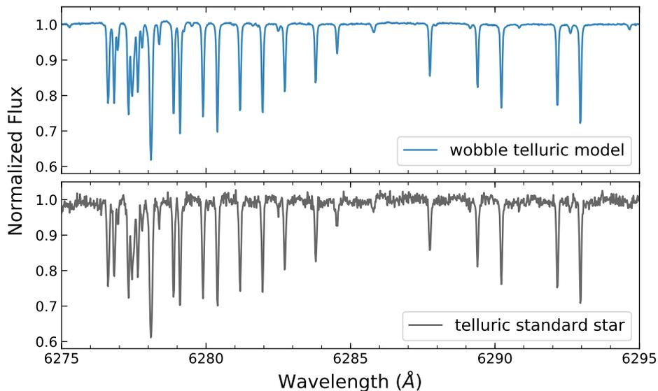
**Figure 8.** Comparison of telluric spectrum derived by *wobble* analysis of 51 Peg spectra (upper panel) and the spectrum observed with a telluric standard star (lower panel) around an H<sub>2</sub>O absorption band. No telluric standard star data was used in determining the *wobble* telluric template. The *wobble* method delivers a very high S/N telluric spectrum with no overhead observing time required.
