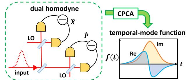
FIG. 1. Conceptual diagram. The input state is a non-Gaussian state in unknown temporal modes. We estimate the temporal mode structure by measuring conjugate quadratures  $\hat{X}, \hat{P}$  by dual homodyne measurement, and processing the data by CPCA.
