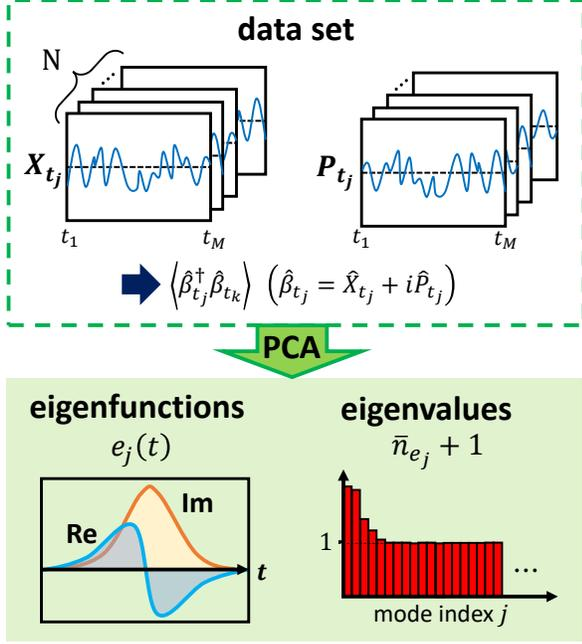
FIG. 2. Schematic of CPCA. For every single shot measurement, we take the quadrature values  $M$  times in  $[0, T]$ . We convert the complex variable  $\hat{\beta}_{t_j}$  into uncorrelated variables by PCA, where we utilize the correlation  $\langle \hat{\beta}_{t_j}^\dagger \hat{\beta}_{t_k} \rangle$  calculated from  $N$ -frame data. From the eigenfunctions and eigenvalues, we can estimate the TMFs of the input states.
