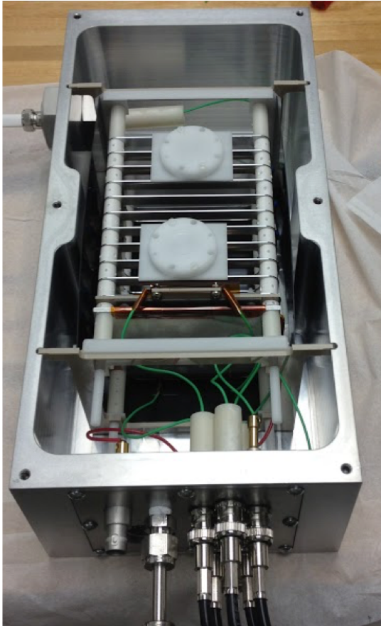
Figure 9: Eight final BEAST TPCs were constructed and deployed. This photo shows the TPC pressure vessel without the lid but with the field cage installed. The feedthrough endplate with HV and gas services connected is visible at the bottom. The 10-kV HV feedthrough for the cathode is visible at the top left. The two white (acetal) disk-like structures contain the ^{210}\text{Po} calibration sources.
