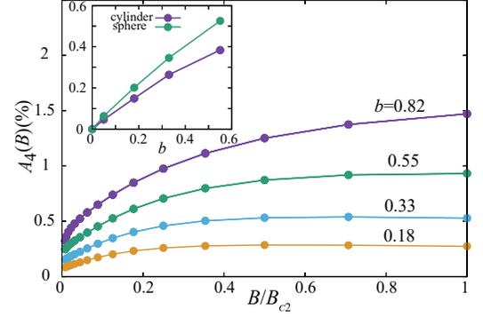
FIG. 28: (color online)  $A_4(B)$  for various  $b$  values for the 3D Fermi sphere case, showing  $\sqrt{B}$ -like increases first and then nearly saturating to a constant as  $B \rightarrow B_{c2}$ . The inset shows  $A_4(B)$  as a function of  $b$ , demonstrating that  $A_4(B) \propto b$  for both 2D cylinder and 3D sphere cases at  $B/B_{c2} = 0.17$ .
