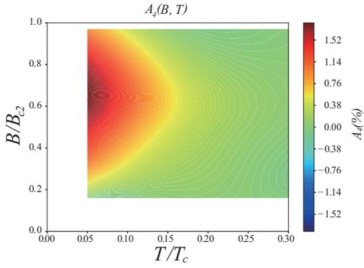
FIG. 14: (color online) Landscape of  $A_4(B, T)$  for  $b = 0.5$  and  $\mu = 0.04$  obtained by using the DOS scaling from Fig. 11.
