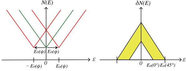
FIG. 3: (color online) Schematic pictures of the Doppler shift. Left: Original V-shape DOS (green) is shifted to two DOS (red) by  $\pm E_D(\phi)$ , producing the increment in ZDOS. Right: Increment  $\delta N(E)$  of DOS due to the Doppler shift as a function of  $E$  obtained by subtracting the two shifted DOS (red) from original DOS (green). A triangle centered at  $E = 0$  forms whose size depends on the field-orientation  $\phi$  through  $E_D(\phi)$ .
