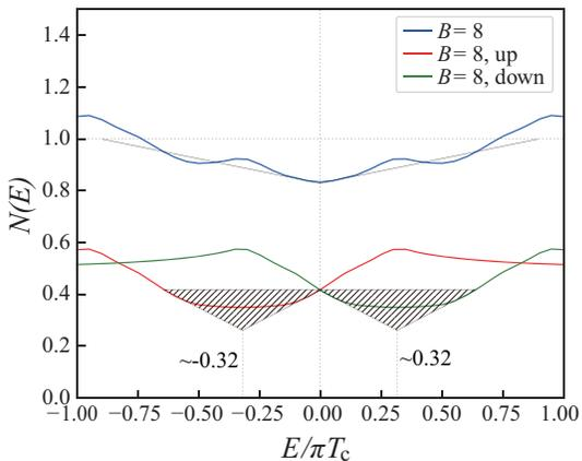
FIG. 12: (color online) Reconstruction of the V-shape DOS  $N(E)$  under PPE. Red and green curves are the spin-resolved DOS and the blue curve is total DOS. To accommodate the excess Pauli paramagnetism due to PPE, the original V-shape  $N(E)$  for spin-up and spin-down are modified to have flat bottoms shown by shaded triangles. Note that in spite of this modification the slope of the original V-shape DOS is preserved under PPE. See the details in the main text.
