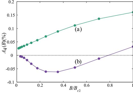
FIG. 26: (color online) Field dependences of  $A_4(B)$  for HLN (a) and full gap (b) as calculated by KPA.  $b = 0.33$ .  $A_4(B) > 0$  for all  $B$  and remains finite when  $B \rightarrow 0$  for the HLN case (b) while in the full gap case (a)  $A_4(B) \rightarrow 0$  as  $B \rightarrow 0$  and changes its sign as  $B$  increases.
