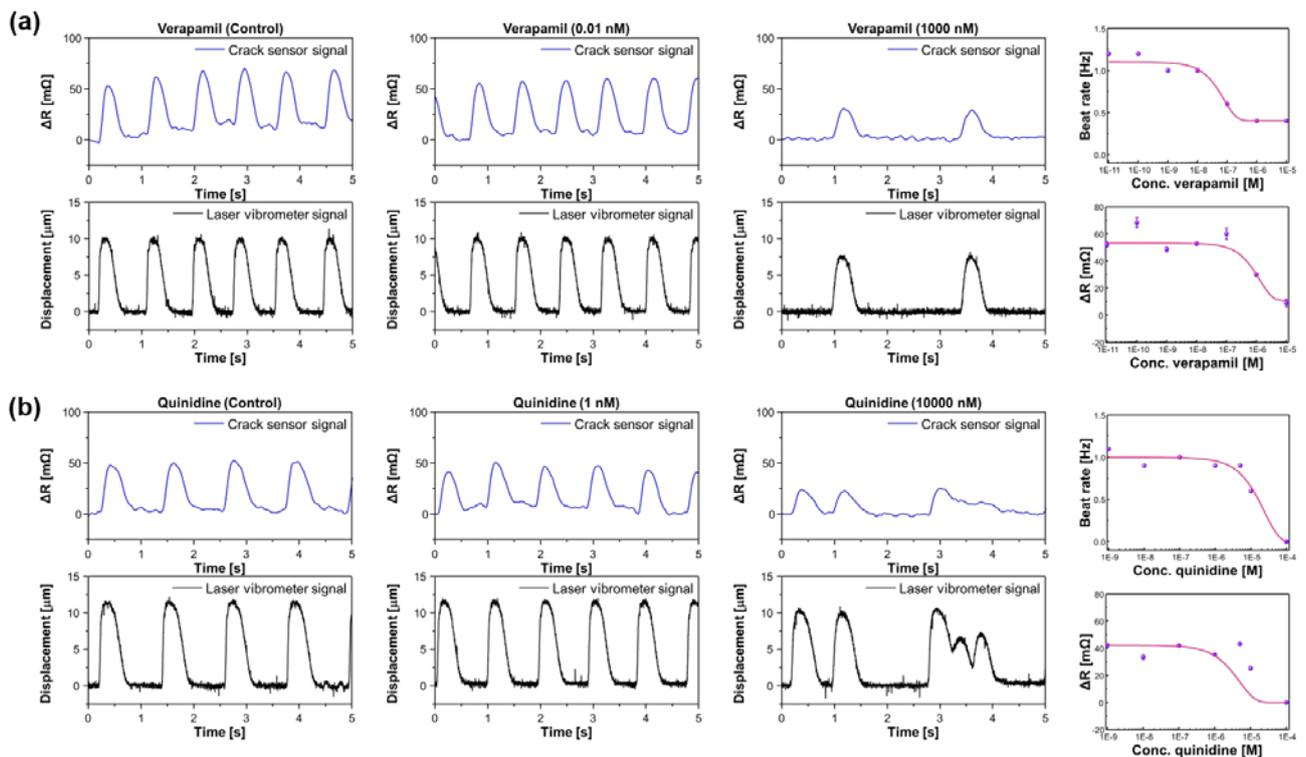
Figure 6. Changes in sensor resistance and cantilever displacement as a function of drug concentration for (a) Verapamil and (b) Quinidine
