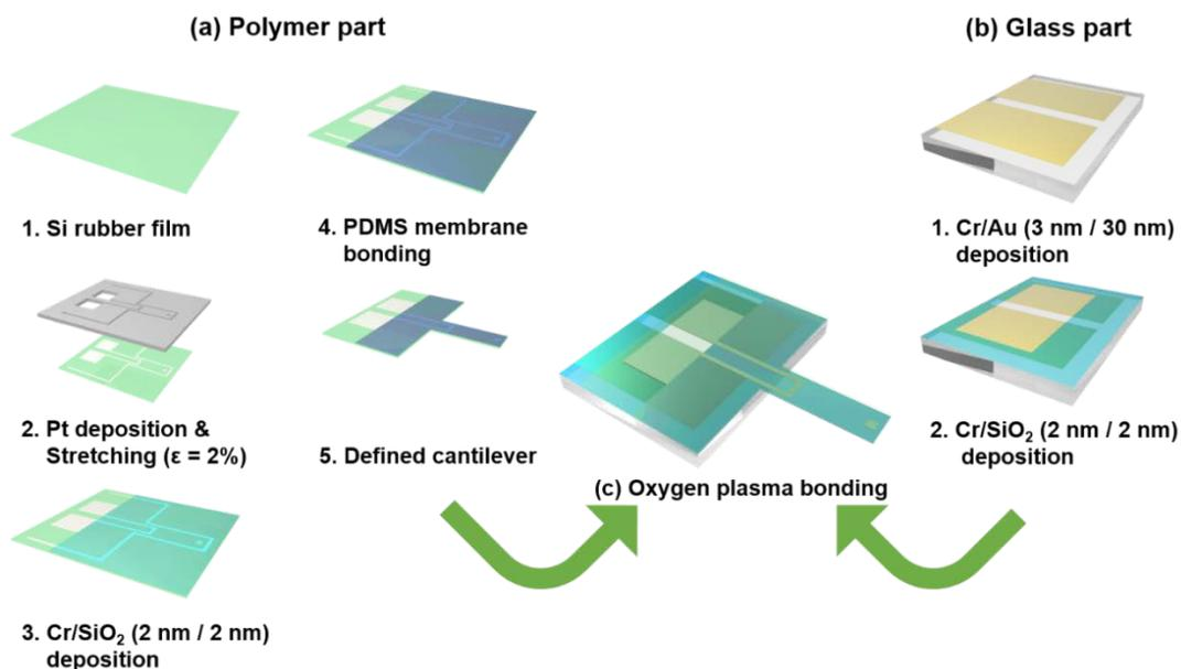
Figure 7. Process flow for the fabrication of the proposed cantilever sensor integrated with a PDMS-encapsulated crack sensor
