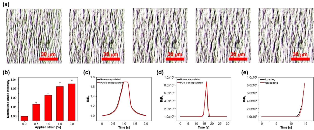
Figure 2. (a) Optical microscope images of the PDMS-encapsulated crack sensor before and after stretching ( $\epsilon = 0, 0.5, 1, 1.5, 2\%$ ). (b) Intensity of cracks according to the applied tensile strain. Resistance changes as a function of strain ranging from (c) 0 to 0.3% and from (d) 0 to 1%, respectively. (e) Hysteresis of the PDMS-encapsulated crack sensor.
