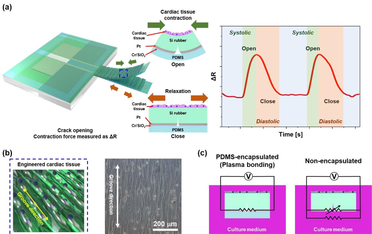
Figure 1. (a) Schematic of a Si rubber cantilever composed of various layers and operation principle of the cantilever sensor integrated with a PDMS-encapsulated crack sensor to measure the contractile force of cardiac cells in liquids. (b) Nano-patterns used to align the cardiac cells on the cantilever surface. (c) Circuit diagrams of two different crack sensors operating in culture media
