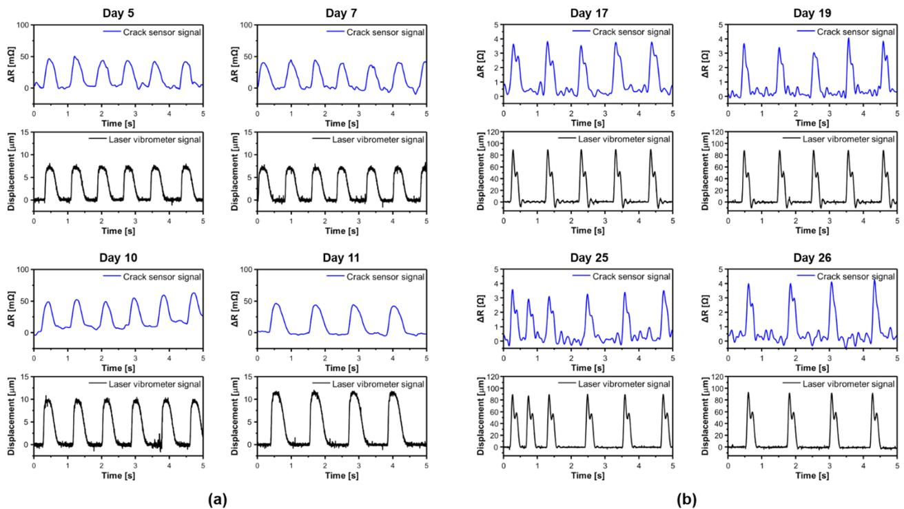
Figure 5. Resistance changes and corresponding displacements of the PDMS-encapsulated crack sensor measured over 26 days
