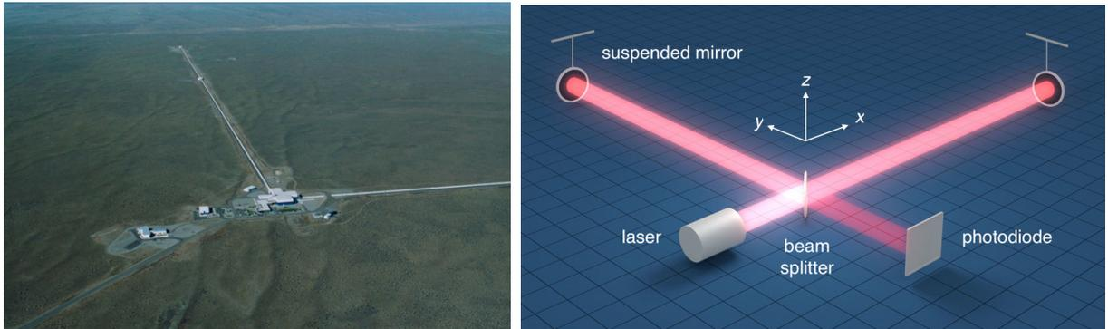
**Figure III.4** *Left panel:* LIGO, Hanford site (USA). The two arms of the interferometer are about four-kilometre long. *Right panel:* Schematic view of the interferometer. A laser beam is split in two, each half-beam is reflected by a suspended mirror, both are recombined, and the resulting superposition is measured by a photo-diode. Adapted from <https://www.ligo.caltech.edu>.
