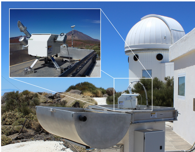
Fig. 1. The solar tracker with the attached optical fibre assembly used to feed sunlight to the SONG spectrograph. The SONG dome and container are seen in the background.
