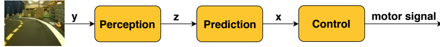
Fig. 11: The pipeline of Gao Wei processes an image y to find the lane, its curvature and possible stop lines. These are further transformed to provide a bird's-eye perspective x to the controller. The controller then follows a pure-pursuit strategy based on the estimated 3D map.
