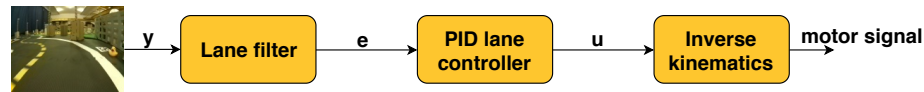
Fig. 14: The ROS-based PID pipeline adapted by Vincent Mai. Images y are processed by the lane detector to estimate position error e for the PID controller. The controller determines the speed and angular velocity commands u and the inverse kinematics node converts these into motor commands.
