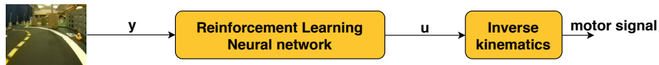
Fig. 15: Reinforcement learning pipeline developed by team JetBrains. Images y are processed by a neural network trained through reinforcement learning. The network computes the speed and angular velocity commands u and the inverse kinematics node converts these into motor commands.
