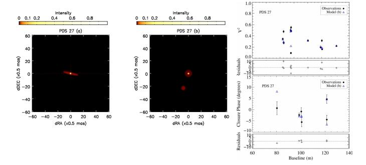
**Fig. 2.** Best-fit geometrical models (a) flattened ring (Red.  $\chi^2 \sim 10$ ) and b) binary (Red.  $\chi^2 \sim 12$ )) are compared with the observed visibilities (V<sup>2</sup>) and closure phases of PDS 27. The black points with vertical error bars are the observed data, and the blue triangles correspond to a representative best-fit model. The two models show a similar fit, and therefore we show model b as a representative fit.
