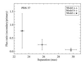
Fig. B.2. Separations and flux ratios of PDS 37 when modelled as binary. The best fit binary models (a, b, c) are presented in Figure 1. All binary models indicate separations of  $\sim$ 22-28 mas which correspond to 42-54 au at the distance of the source. The flux ratios are characterized by a large uncertainty but we observe decreasing flux ratios with increasing separations.
