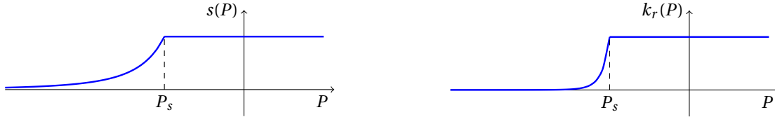
Figure 2: Saturation and relative permeability in terms of the pressure: the Brooks and Corey model.
