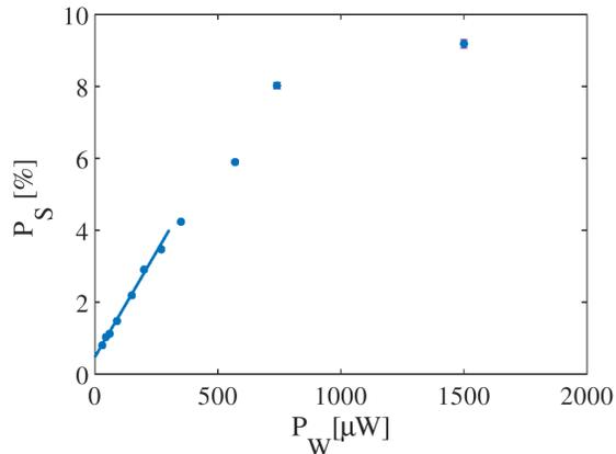
FIG. 5: Stokes creation probability,  $P_S$ , as a function of the write pulse power,  $P_W$ . A linear fit of the data points at lower  $P_W$  is also shown. The fitting curve intercepts the y axis at  $P_S = 0.5\%$ .
