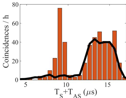
FIG. 6: Time resolved Stokes-anti-Stokes coincidence histogram (red bars) plotted together with the accidental coincidence histogram (solid curve) for  $P_W = 90 \mu\text{W}$ , corresponding to  $P_S = 1.6\%$ .
