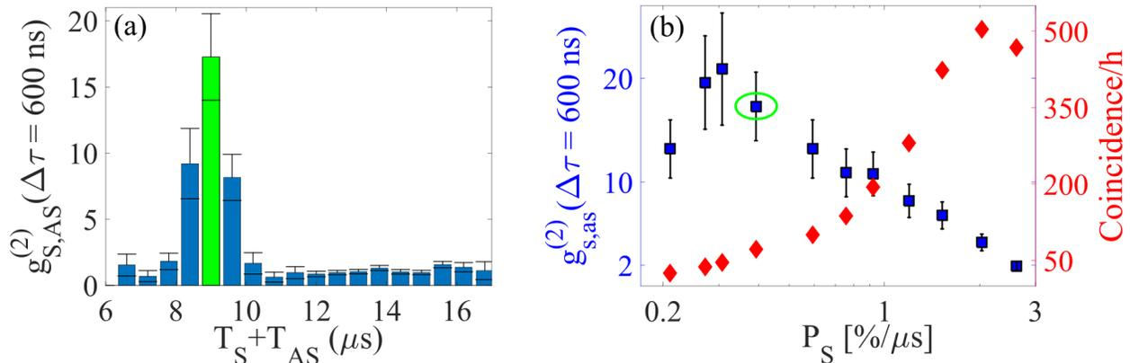
FIG. 2: (a) Typical  $g_{S,AS}^{(2)}$  histogram as a function of the  $T_S + T_{AS}$  time, with a time-bin size of 600 ns. The write pulse power  $P_w$  is  $90 \mu\text{W}$ , corresponding to a Stokes creation probability  $P_S = 0.4 \%/ \mu\text{s}$ . (b)  $g_{S,AS}^{(2)}$  (blue squares) and coincidence rate (red diamonds) vs Stokes creation probability. Both quantities refer to a time-bin size of 600 ns. The errorbars are calculated assuming Poissonian statistics.
