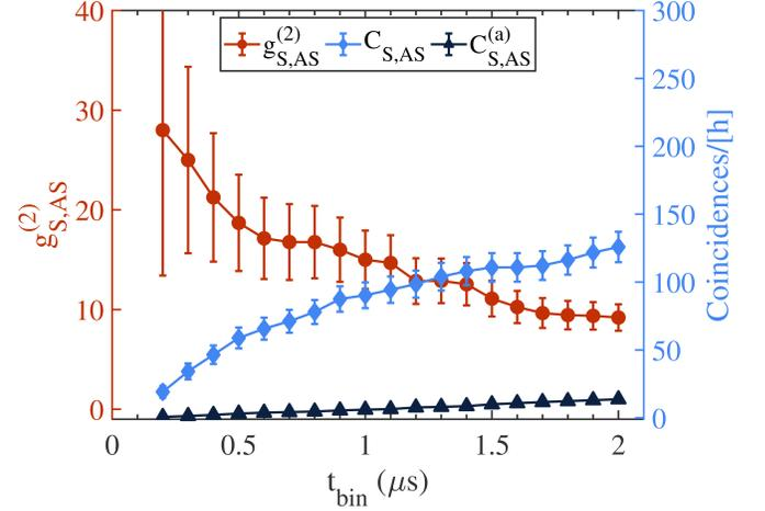
FIG. 10: The cross-correlation function  $g_{S,AS}^{(2)}$  (red dots), the coincidences per hour  $C_{S,AS}$  (blue diamonds) and the accidental coincidences per hour  $C_{S,AS}^{(a)}$  (black triangles) as a function of the coincidence detection window width  $t_{bin}$ .
