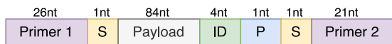
Fig. 3: Format of the oligos - S denotes the sense nucleotide which determines whether a strand is reverse complemented when sequenced. P is a parity check nucleotide while the ID is an identifier of the image so to be distinguished from other data that may be stored. Payload contains encoded chunks, including specific headers.
