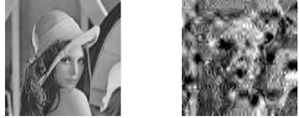
Fig. 5: Visual results for two different cases at 2.68 bits/nt: Reconstruction using the most frequent oligos (left) and random selection (right). For the left image the PSNR value is only due to the error inserted by the quantization process as we have managed to get a reconstruction without any sequencing noise.
