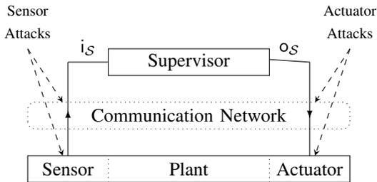
FIGURE 1: Supervisory control of cyber-physical systems. At each time, the plant sends a sensing symbol, which will be corrupted by  $o_P$  to the supervisor. Then, the supervisor replies to the plant with an actuating symbol  $i_P$ . A plant transition can only happen if the pair  $(i_P, o_P)$  matches the transition's label. In practice, the symbols  $o_P$  and  $i_P$  may be revised by malicious attackers, causing the plant to make transitions not allowed by the supervisor.
