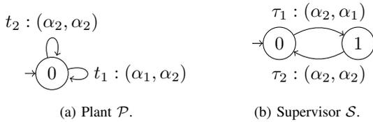
FIGURE 3: Example of supervisory control of FST plants.
