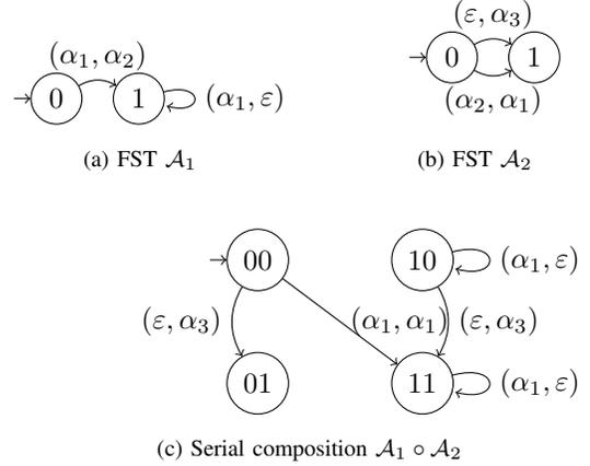
FIGURE 5: Example for serial composition of FSTs.
