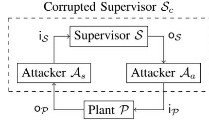
FIGURE 4: Block diagram for supervisory control under sensor and actuator attacks. The serial composition of  $\mathcal{A}_a$ ,  $\mathcal{P}$ , and  $\mathcal{A}_s$  in the dashed box form the corrupted supervisor. The executions of the plant  $\mathcal{P}$  in this control loop is derived by its loop composition with the corrupted supervisor.
