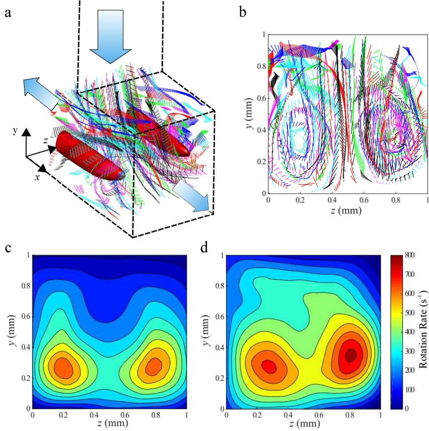
Fig. 6. (a) Visualization of the measured rod trajectories. Solid lines show the measured 3D orientation of the rods. Colors indicate individual particles. Vorticity isosurfaces ( $\omega = 3000s^{-1}$ ) are from the CFD simulation. (b) View of the experimental fiber orientations in the yz plane. (c) Contour map of the particle rotation rate ( $s^{-1}$ ) expected from the simulation. (d) Measured 3D particle rotation rate.
