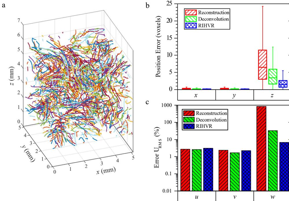
Fig. 2. (a) Smoothed 3D particle trajectories extracted from a synthetic hologram using RIHVR. (b) Localization error of tracked particles relative to their true locations. (c) Error in the RMS velocity components of the three test methods compared to ground truth.
