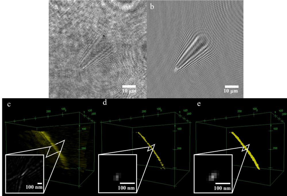
Fig. 1. (a) Recorded holographic image of a 90 nm Ag nanowire. (b) Hologram after image enhancement. (c) Volumetric reconstruction of the sample using the deconvolution method. (d) Reconstruction using RIHVR with sparsity ( $\ell^1$ ) regularization. (e) Reconstruction using RIHVR with fused lasso (FL) regularization. For visualization, (c) uses the intensity as the transparency alpha value while (d) and (e) show all non-zero values at equal intensity.
