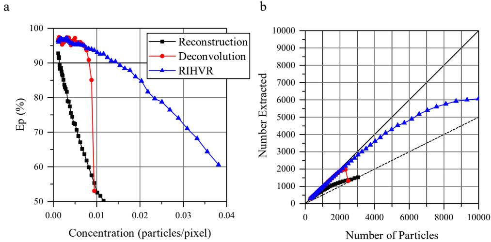
Fig. 3. (a) Extraction rate for each method for increasing particle concentrations. (b) The number of particles which can be accurately extracted is higher for RIHVR than the other methods. Solid line is 100% EP, dashed line is 50%.
