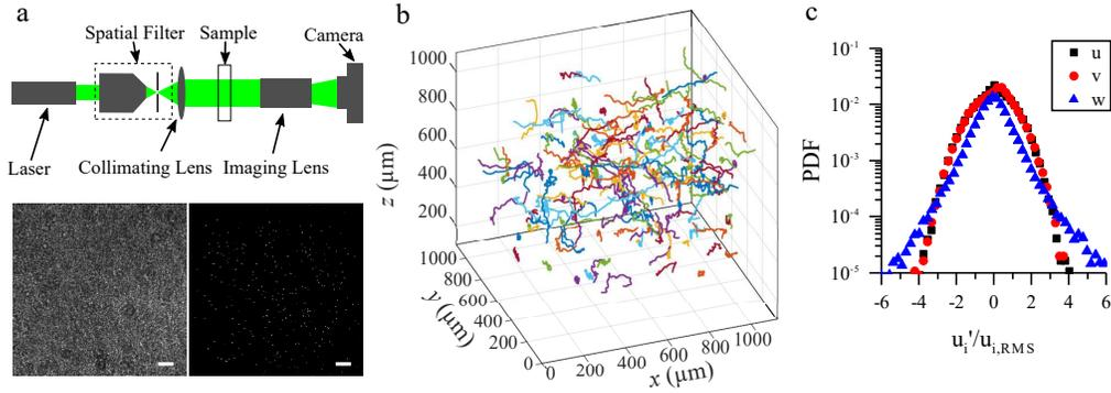
Fig. 4. (a) DIH imaging system, recorded hologram, XY projection of processed reconstruction. Scale bars are 100  $\mu\text{m}$ . (b) Subset (25%) of tracked particles. (c) PDF of velocity fluctuations in each direction. The  $w$  distribution has longer tails and a sharper peak but is not substantially wider than the other two components.
