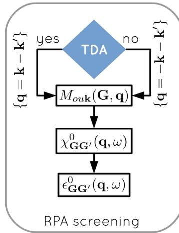
Figure 10: Flowchart for the calculation of the RPA dielectric function.
