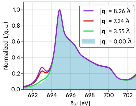
Figure 4: Normalized loss function for the F K edge of LiF with increasing values of momentum transfer. All spectra are normalized at the main peak. Spectra are broadened by a Lorentzian function with full-width at half maximum of 0.5 eV.
