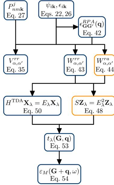
Figure 1: Schematic workflow of BSE calculations in `exciting`. Quantities that are calculated if the Tamm-Dancoff approximation is lifted, are shown in yellow.
