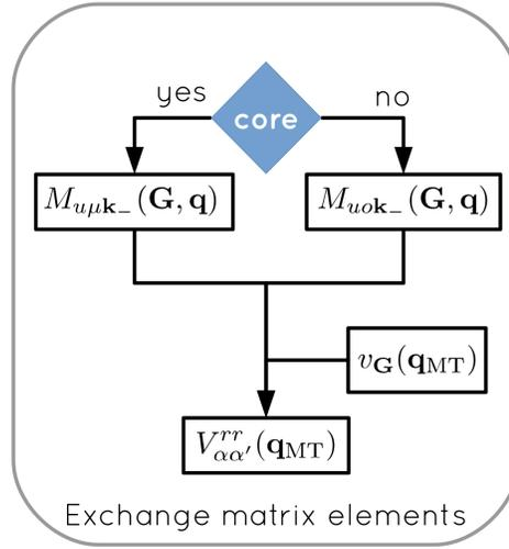
Figure 12: Flowchart for the calculation of the matrix elements of the exchange interaction.
