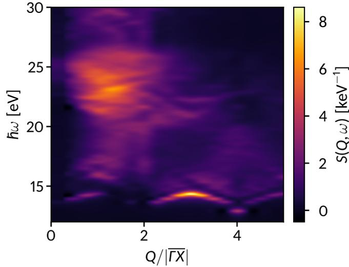
Figure 2: Dynamical structure factor of LiF as a function of the energy loss (vertical axis) and the momentum loss (horizontal axis). The momentum loss is chosen along the  $\Gamma$ - $X$  direction until the border of the 5th Brillouin zone.
