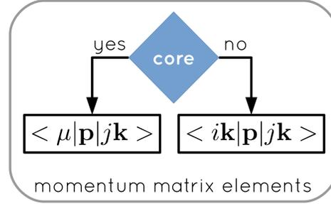
Figure 9: Flowchart for the calculation of momentum matrix elements. The blue triangle indicates the if-condition, where the code checks whether a core-level calculation shall be performed.
