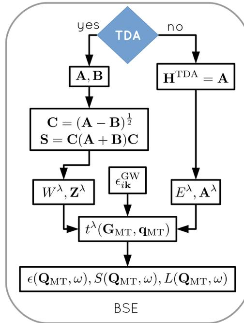
Figure 13: Flowchart for the diagonalization of the BSE Hamiltonian and the construction of the dielectric function.
