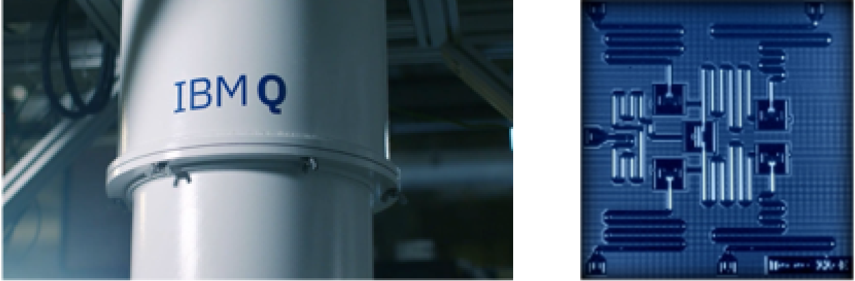
FIG. 9. Dilution refrigerator housing the superconducting quantum hardware (left) and the IBM QX2 quantum chip comprised of five qubits and radio-frequency couplings (right).
