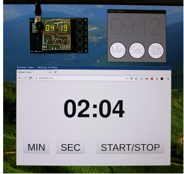
Figure 11. Timer applications: the hardware application built with ClaSH is on the top left. The top right shows the desktop application built using Yampa and the at bottom the web application built using threepenny-gui . All are synthesized from the same CFM.
