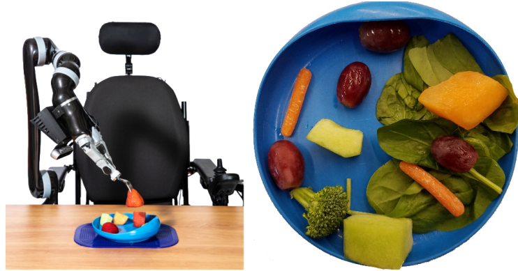
Fig. 1: Left : A robot acquiring a food item from a plate. Right : A plate cluttered with food items. Food items can be isolated, near a wall (i.e., the edge of a plate) or another food item, or stacked on top of other food items.
