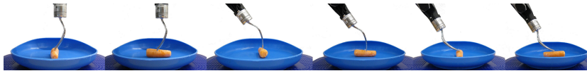
Fig.3: Three macro actions: VS: vertical skewer ( two on the left ), TV: tilted skewer with vertical tines ( two in the middle ), TA: tilted skewer with angled tines ( two on the right ). Each macro action has two fork rolls ( 0^\circ and 90^\circ ).
