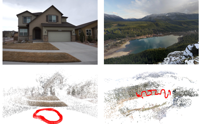
Figure 6. Left: Our method successfully reconstructs the Street dataset [33] without prior calibration. Right: Despite only observing distant features, our method is able to reconstruct camera poses from the Rattlesnake dataset. Reconstructed camera frustums are shown in red.
