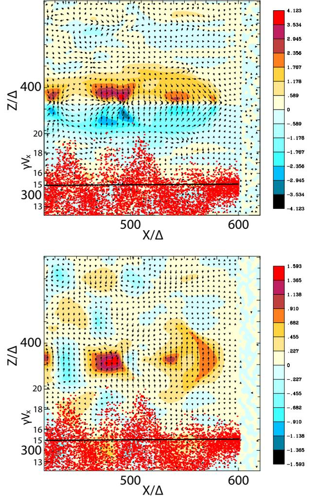
**Figure 6.** Top panel: Contours of  $B_y$  with arrows of  $E_{x,z}$ . Bottom:  $E_x$  with arrows indicating  $B_{x,z}$ . The  $x - \gamma v_x$  distribution of jet electrons at  $t = 500 \omega_{pe}^{-1}$  (a) is overplotted in red. Some jet electrons are accelerated up to  $v_x \gamma = 20$  above the initial  $v_x \gamma = 15$  (the black line) in the phase space. The scale for the phase-space is indicated with small digits at the left axis.
