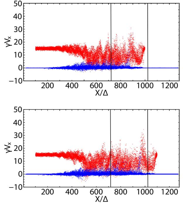
**Figure 4.** Phase-space ( $x - \gamma V_x$ ) distribution of jet (red) and ambient (blue) electrons at  $t = 900 \omega_{pe}^{-1}$  (top) and  $t = 1000 \omega_{pe}^{-1}$  (bottom). The two vertical lines show the regions for which Fig. 3 displays the 3D magnetic-field vectors.
