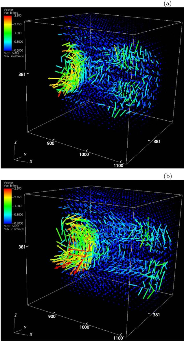
**Figure 3.** Magnetic-field vectors within a cubic section of the simulation grid ( $820 < x/\Delta < 1120$ ;  $231 < y/\Delta, z/\Delta < 531$ ) at time  $t = 900 \omega_{pe}^{-1}$  (a) and at  $t = 1000 \omega_{pe}^{-1}$  (b). To illustrate the magnetic field inside the jet, the plots show the rear half of the jet with cut in the  $x-z$  plane ( $381 < y/\Delta < 531$ ).
