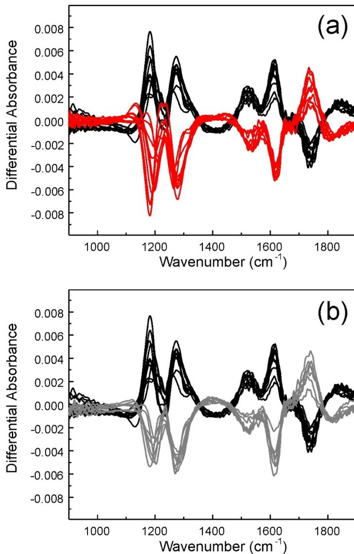
**Figure 4:** (a) CD spectra acquired for two opposite plasmonic enantiomers (black and red lines, respectively) for different azimuthal angles in steps of 20°; (b) CD spectra acquired for the same plasmonic enantiomer after flipping the sample with respect to the propagation direction of the excitation beam (black and grey lines, respectively, the black lines represent the same data as those in panel a) for different azimuthal angles in steps of 20°.
