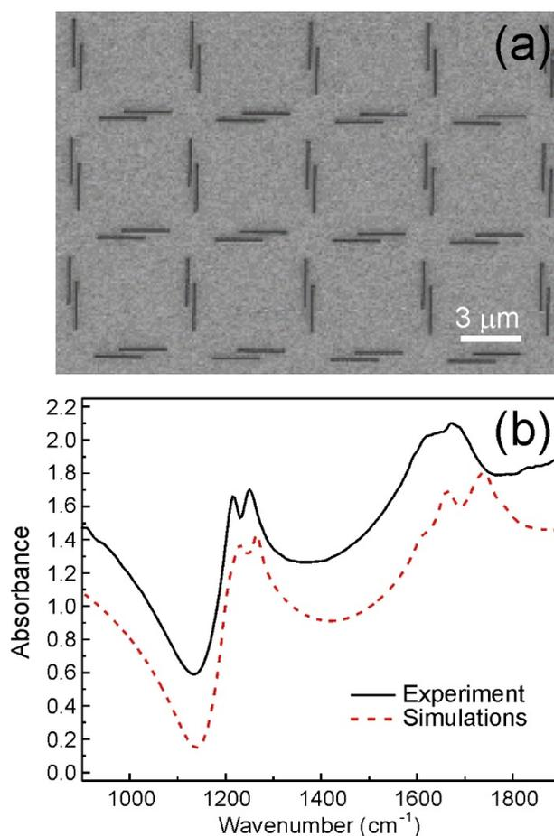
**Figure 3:** (a) Representative SEM image of the square slit array with 6  $\mu\text{m}$  pitch (the widths of the slits and the gap between them are 200 nm and 150 nm, respectively, as in the previous case); (b) transmission FTIR spectrum acquired with a quasi-collimated source (incidence half angle about  $2^\circ$ ) and the associated RCWA simulations obtained by averaging over the same range of angles.
